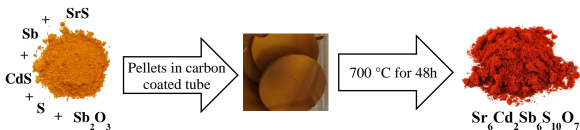
Figure 4.5 : Diagram of the solid-state synthesis of \text{Sr}_6\text{Cd}_2\text{Sb}_6\text{S}_{10}\text{O}_7
