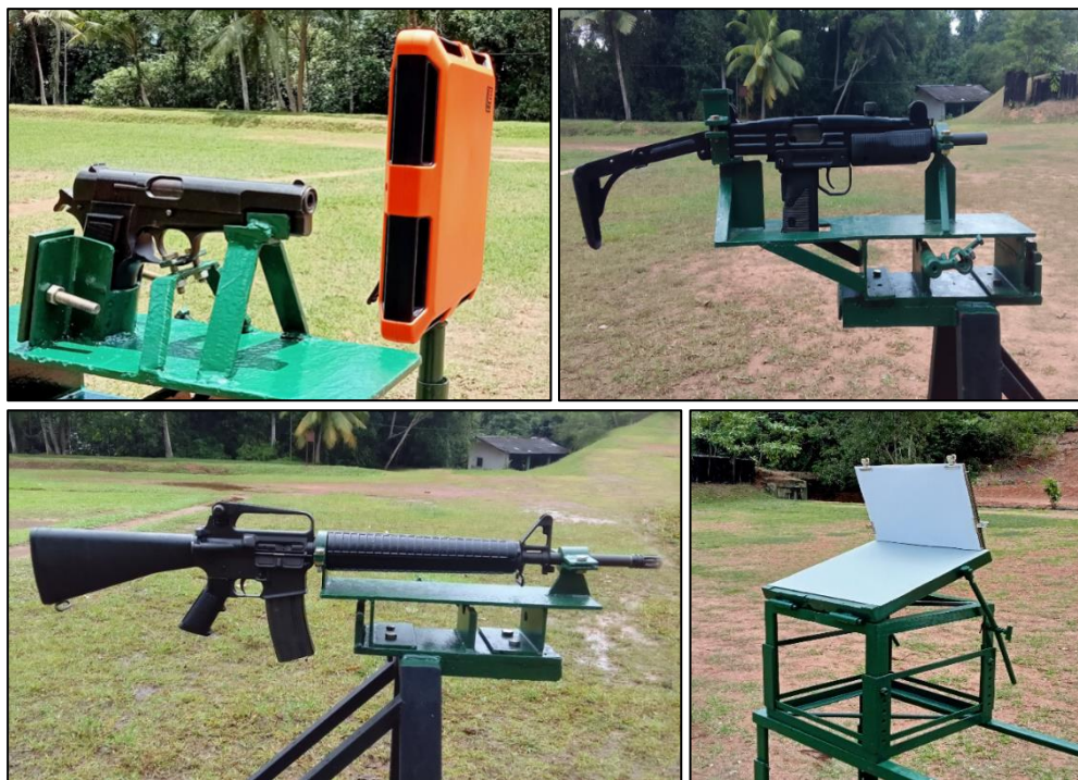
Figure 2: Photographs of the gun mounts and target holder used during the study.
