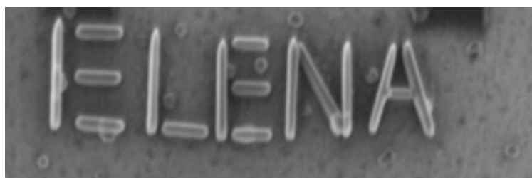
Fig 1.1.1. ELENA \text{Si}(\text{OEt})_4 deposits on Au(111) done with Clone 1 MeRiT column at Zeiss GmbH, Rossdorf, Germany
