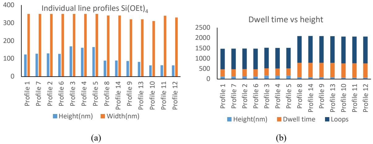
Fig 7.3.3.2.3. Height and width of the individual line profiles (a) and height versus dwell time (b) of 12 hours old structures
