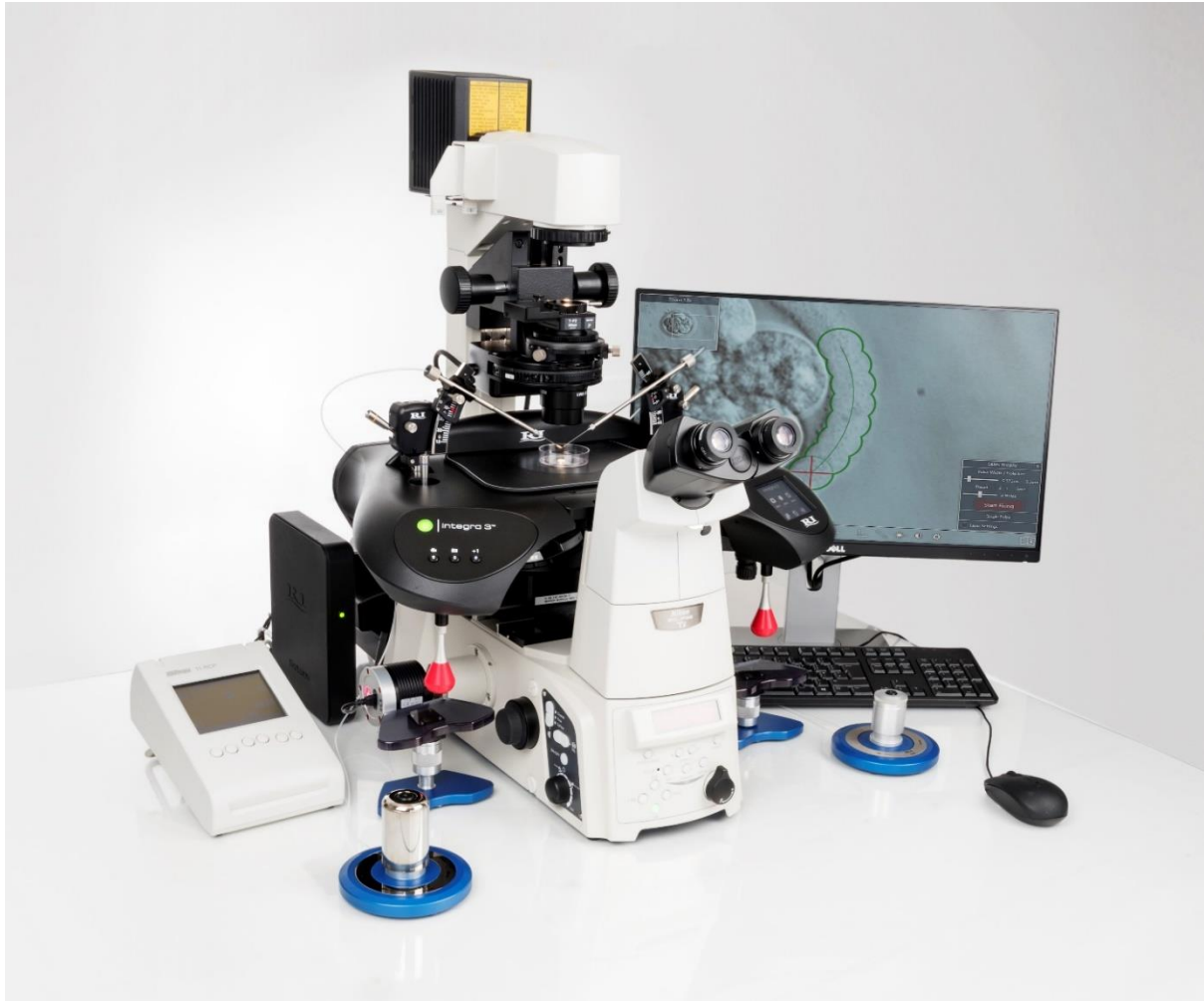
Figure 1.4. Typical embryology laboratory set up for biopsy including microscope, ICSI holdings and syringes, laser, and PC with laser and biopsy software. Image courtesy of CooperSurgical Fertility and Genomics Solutions.
