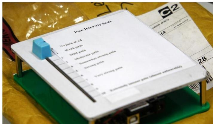
Figure 2.2. Custom built pain recording device (linear potentiometer) to record rating of pain every 2s.
