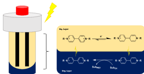
Scheme 4.8 Proposed mechanism for biphasic electrocatalysis using an IKA Electrasyn.
