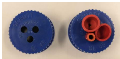
Figure 3.18 New lid design for \gamma -generation RFB design.
