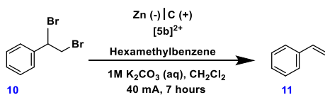
Scheme 4.12 Biphasic electrocatalysis using Zn as a sacrificial cathode.
