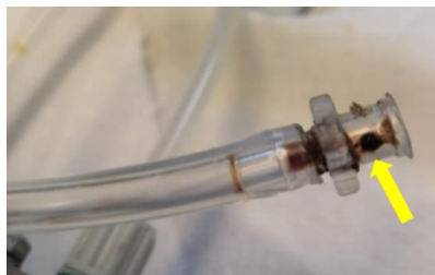
Figure 3.6 Blockage of tubing fitting due to precipitation.
