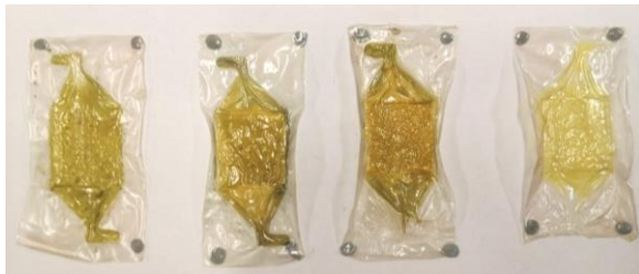
Figure 3.25 Evidence of fouling on AEMs used in FCN-based cell tests.
