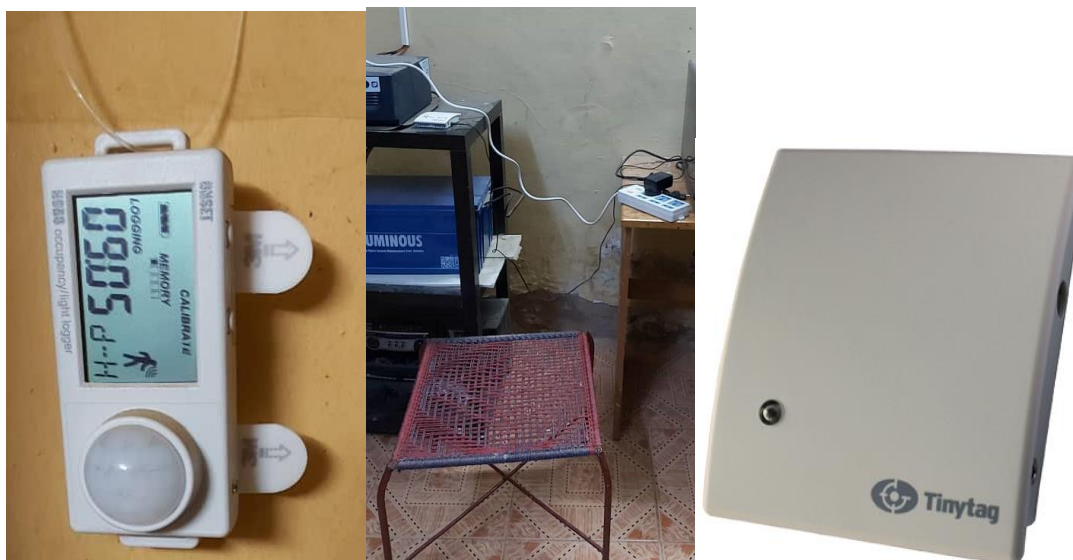
Figure 3.4 Left: A photo of the PIR Hoboware logger used showing it had detected motion. Middle: the carbon logger installed in the case study T1. Right: a photo of the carbon logger
