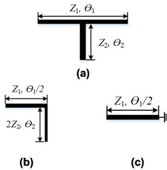
**FIGURE 2.** Equivalent circuit for the stub-loaded resonator. (a) stub-loaded resonator. (b) even mode. (c) odd mode.
