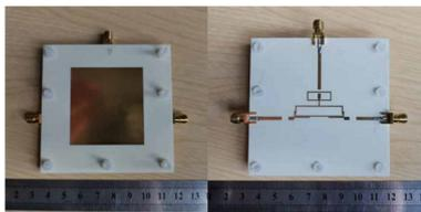
FIGURE 15. Fabricated antenna.
