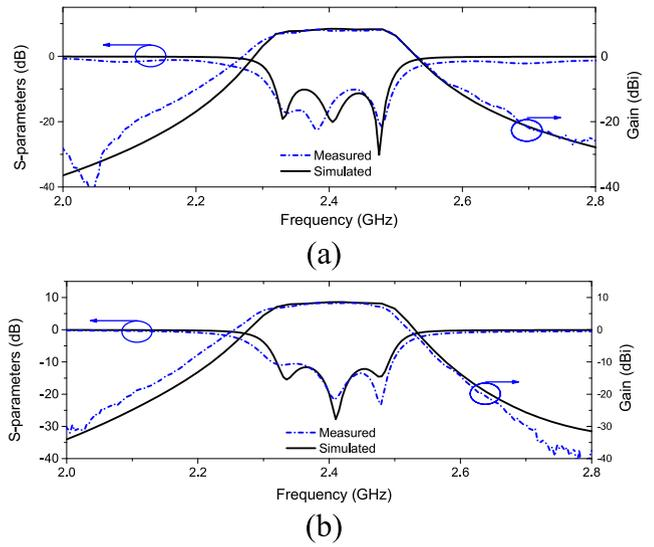
**FIGURE 6.** Simulated and measured *S*-parameters and gains of the dual-polarized antenna. (a) Even-mode driven. (b) Odd-mode driven.
