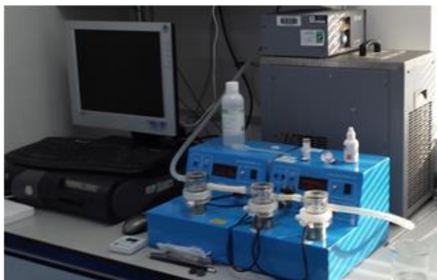
Figure 2.4 - Oxygen electrode arrangement. Oxygen electrode in the bottom right containing 2 chambers connected to thermostatically controlled water bath and pump. Voltage data recorded by computer on the left.
