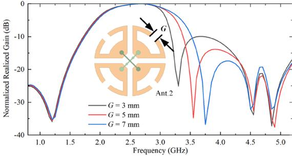
Fig. 8. Ant.2's simulated normalized gain under various  $G$ .
