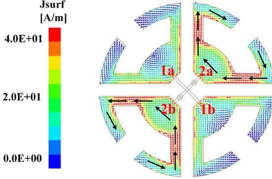
Fig. 7. Simulated current distribution on Ant.2 at 3.5 GHz
