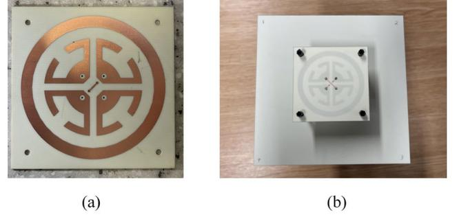
Fig. 10. Fabricated prototype of the proposed antenna.
