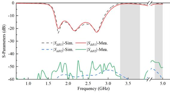
Fig. 11. Measured and simulated  $|S_{dd11}|$  and isolation.
