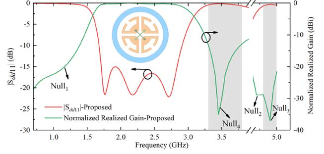
Fig. 9. The normalized gain and  $|S_{dd11}|$  obtained from HFSS software.
