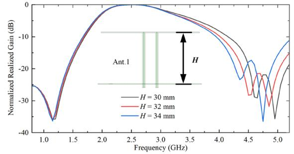
Fig. 5. Ant.1's simulated normalized gain under various  $H$ .
