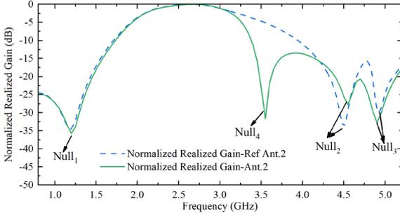
Fig. 6. Simulated normalized realized gain of the Ant.2 and Reference Ant.2.
