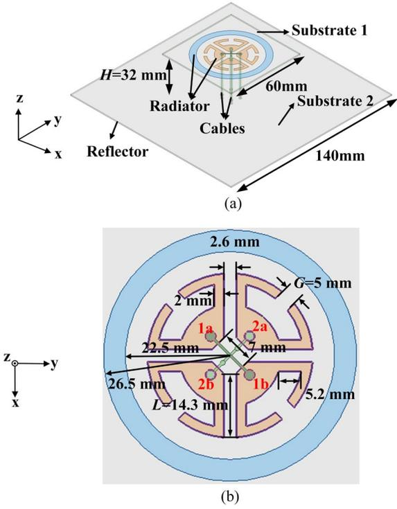
Fig. 1. The simulated antenna geometry. (a) 3D view, and (b) top view.
