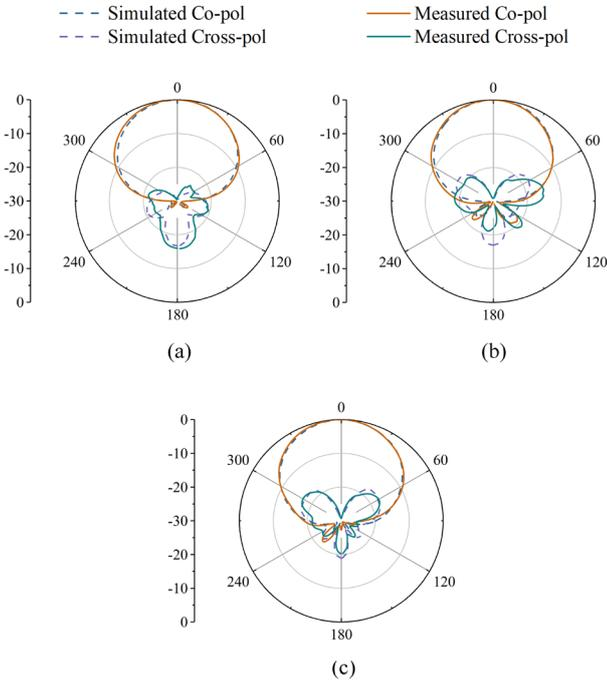
Fig. 13. Measured and simulated normalized radiation patterns of the proposed antenna at (a) 1.7 GHz, (b) 2.2 GHz, and (c) 2.7 GHz.
