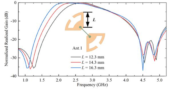
Fig. 4. Ant.1's simulated normalized gain under various  $L$ .
