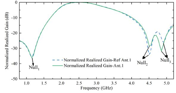
Fig. 3. Simulated normalized gain of the Ant.1 and Reference Ant.1.
