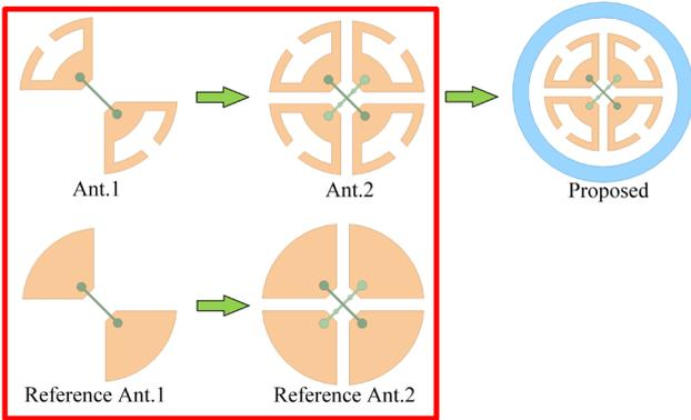
Fig. 2. Evolution of the proposed antenna.
