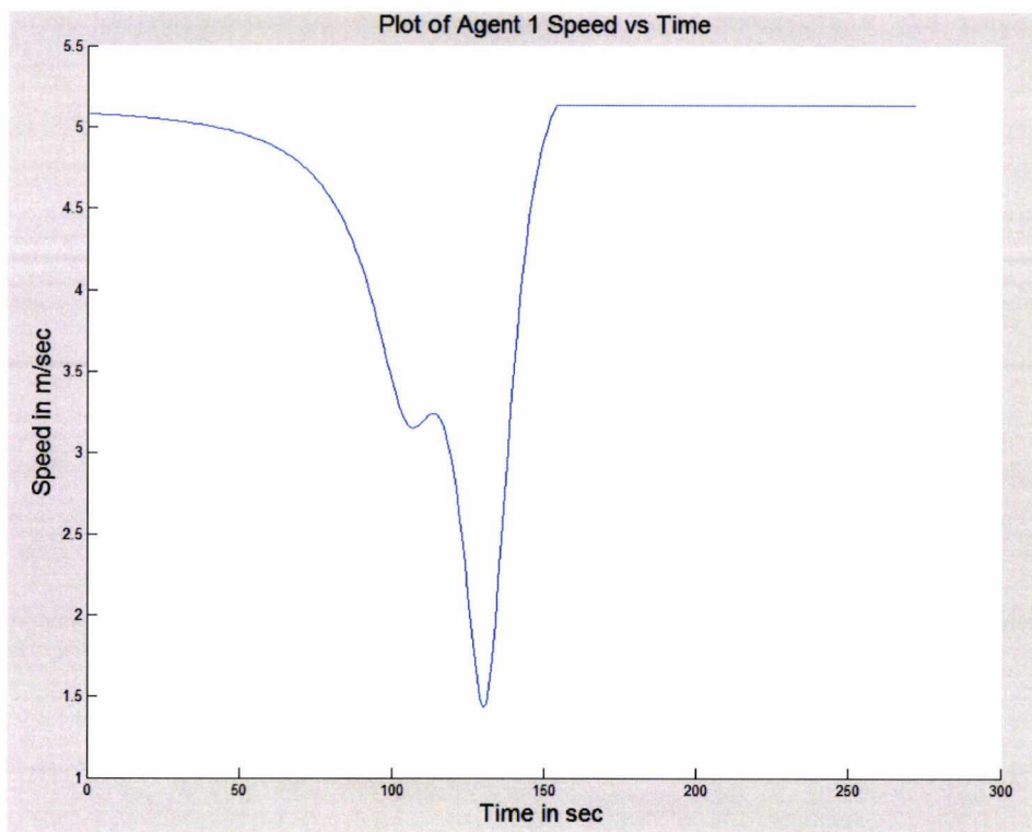
Figure 5-18: Autonomous Vehicle Speed Variation due to the Dynamic Obstacle vs Time when the Autonomous Vehicle is guided by the AWSPPF algorithm.
