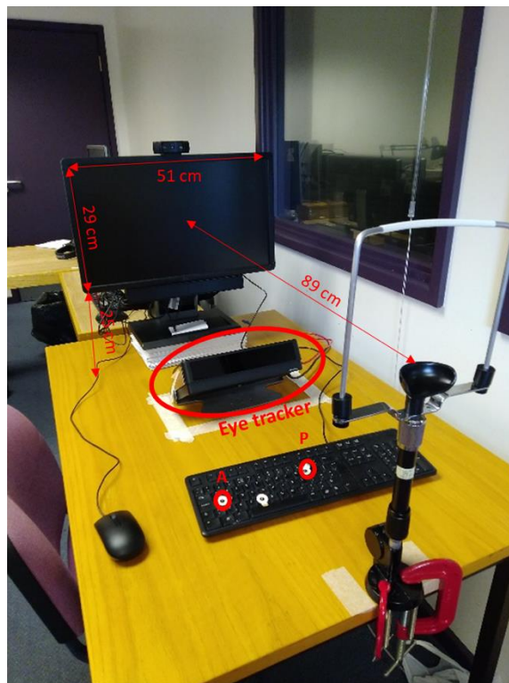
Figure 3.2 Visual training experimental setup. Experimental setting including computer, eye tracker and headrest.
