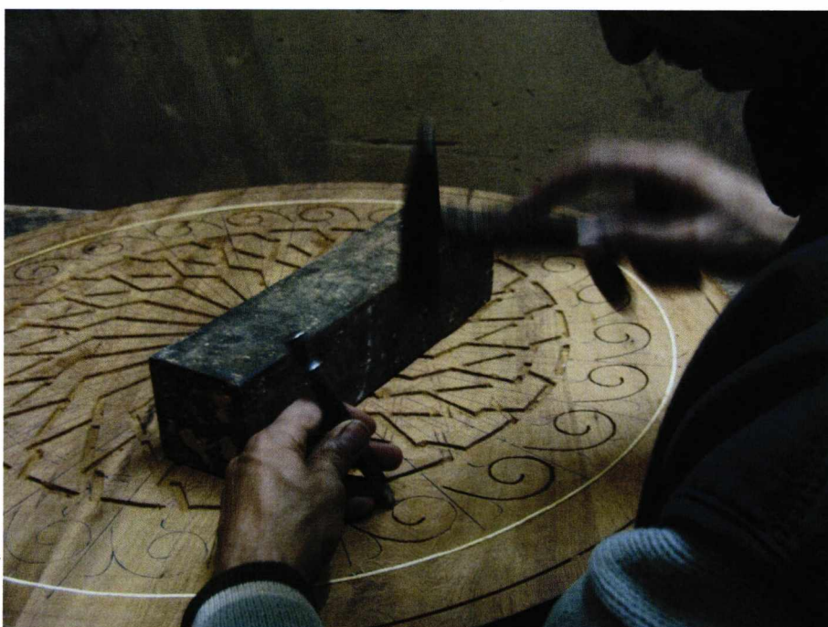
Plate 6.7: After the design has been drawn out on the base-board, the mribâr and a hammer are used to hammer out the design.
