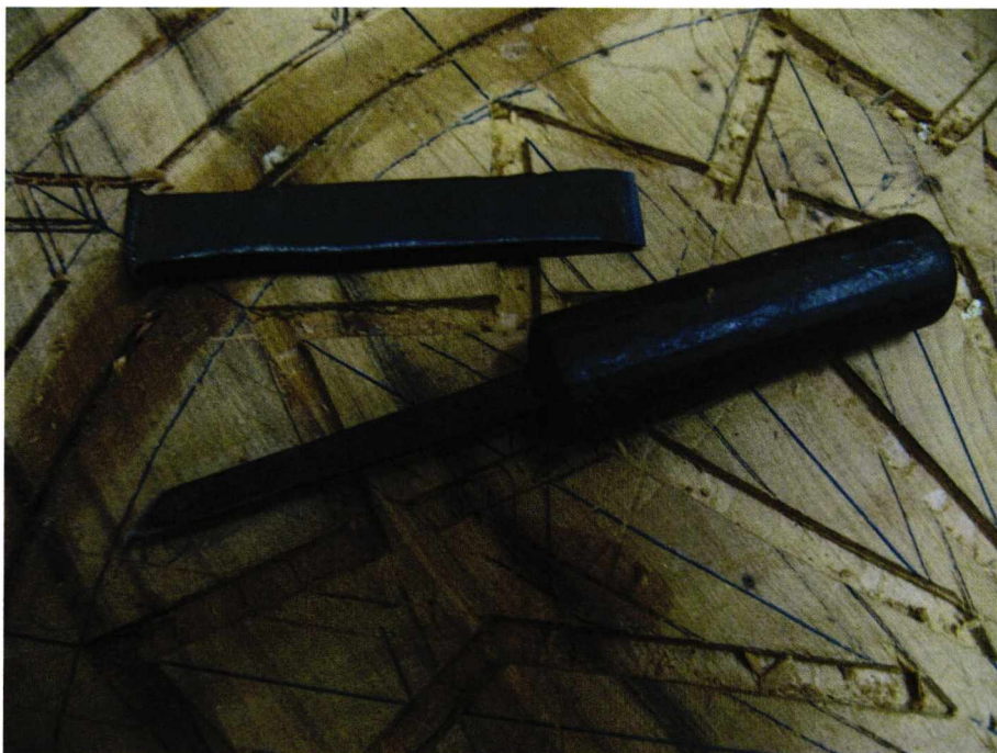
Plate 6.6: The mribâr (top) and bominqar (bottom), the two main tools used for inlay work.
