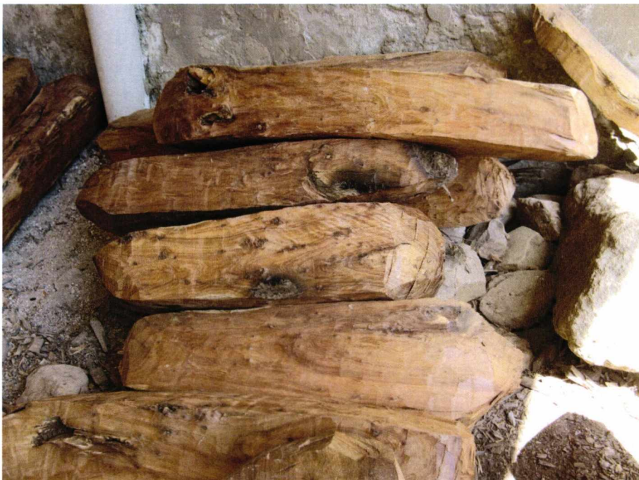
Plate 4.3: Bildi beams in a stack waiting to be sold in a closed depot in Essaouira. The beams are around 90cm in length. Note the rich red colour characteristic of bildi wood, and the twists and knots within the wood that make it difficult to work.
