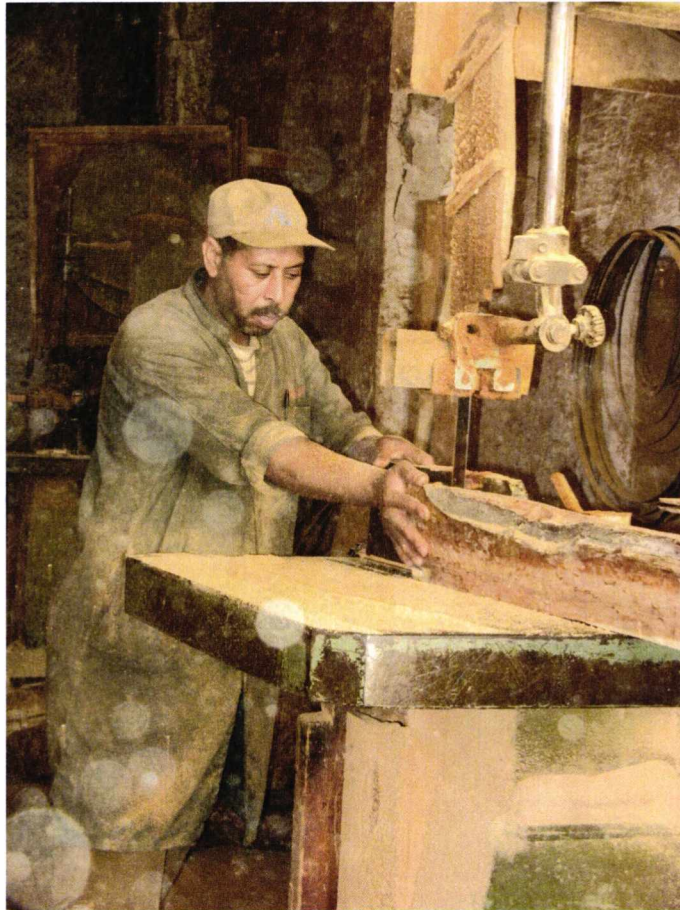
Plate 4.8: Sawmill worker cutting a beam into planks with the bandsaw. Note the blemishes on the photo caused by the high levels of wood dust in the air. There is no health and safety equipment.
