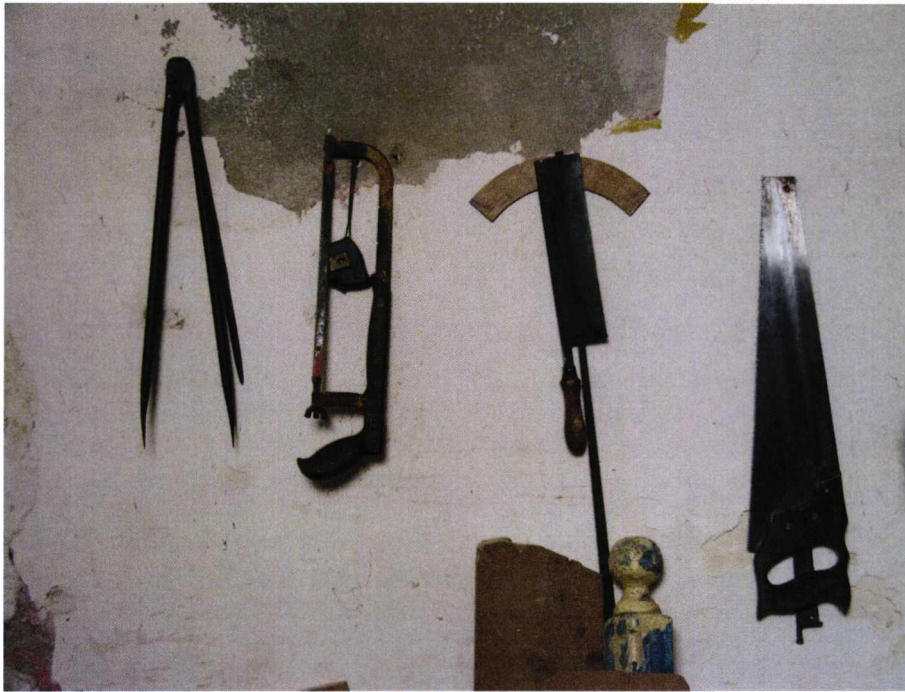
Plate 5.10: Larger hand tools hanging on nails on the wall. From the left: large compasses for drawing designs, hacksaw and tape measure, tenon saw and template, general purpose saw.
