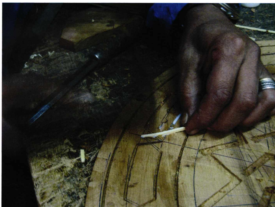
Plate 6.11: The citron strip is hammered into the groove.
