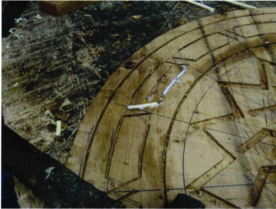
Plate 6.12: The citron strip is cut to the correct length with a chisel, and more glue applied to the next section to be infilled.
