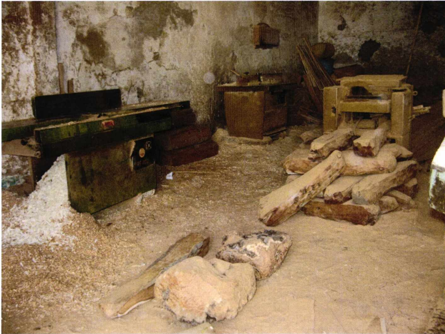
Plate 4.6: Sawmill, showing three table planing machines. The piles of beams and burl on the floor belong to different artisans and are waiting to be cut. 18/11/05.
