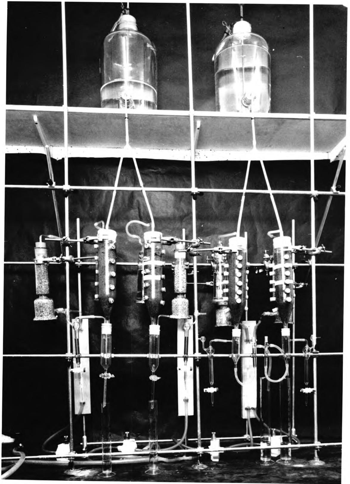
Figure 2.3. Apparatus used for studying microbiological processes in soil by means of the continuous flow method.
