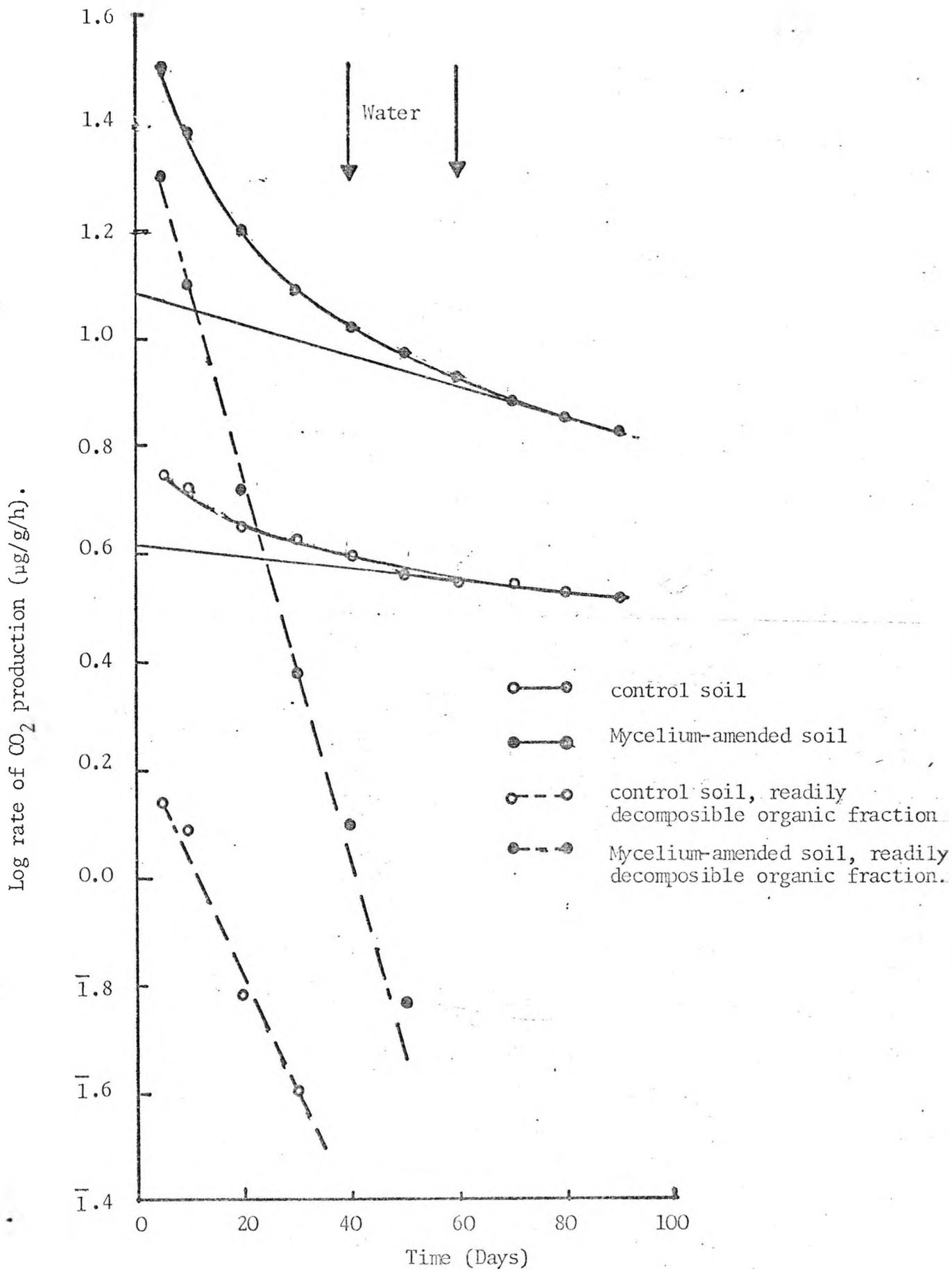
Figure 4.7. Evolution of CO<sub>2</sub> from mycelium-amended and control soils under aerobic conditions during continuous flow of ammonium-sulphate solution (100µg NH<sub>4</sub> - N/ml). At day 40 the flow was changed to one of water and at day 60 the flow of (NH<sub>4</sub>)SO<sub>4</sub> was restored. Other details as in Figure 4.1.
