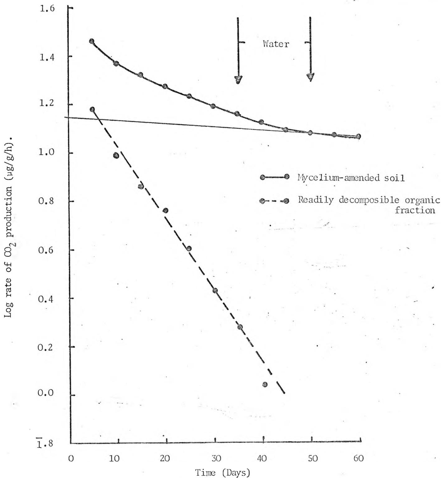
Figure 4.5. Evolution of CO<sub>2</sub> from mycelium-amended soil under aerobic conditions during continuous flow of glucose solution (0.1%, w/v). At day 35 the flow was changed to one of water and at day 50 the glucose flow was restored.
