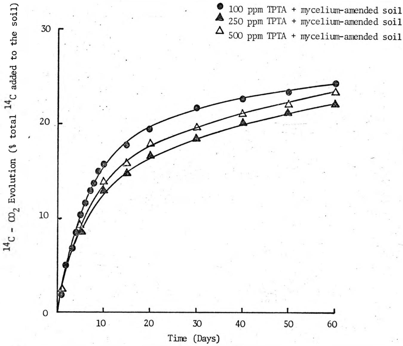
Figure 3.4.9. Release of  $^{14}\text{CO}_2$  from  $^{14}\text{C}$ -labelled mycelium during the continuous flow of aqueous fentin acetate through soil columns; aerobic incubation conditions.
