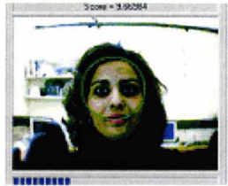
Figure 3.1: FaceIt SDK detects human faces by finding the area enclosed by the circle
