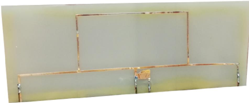
FIGURE 4.20: Finalised GAA Prototype.
