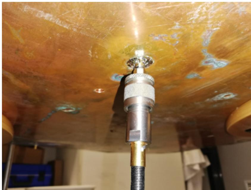
FIGURE 4.23: VNA coaxial connection to SMA pin underneath the ground plane.
