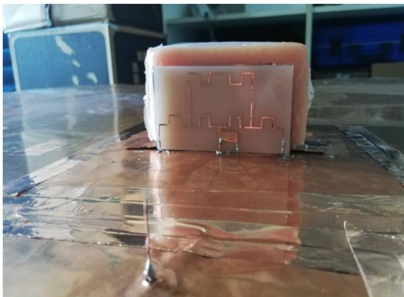
FIGURE 5.16: GAA miniaturisation prototype on body-phantom roasted pork.
