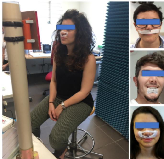
FIGURE 2.16: Experimental setup for epidermal tags characterization and breath detection by the help of some volunteers [82].
