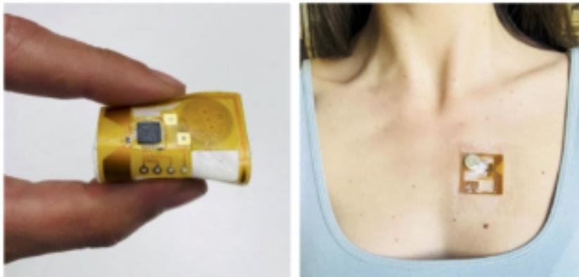
FIGURE 2.3: Prototype of the epidermal board with two-way discrete impedance tuning and its application on the skin by 5  $\mu\text{m}$  polyurethane film [44].
