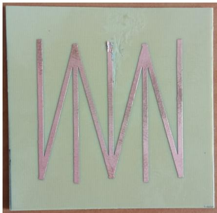
FIGURE 6.10: Folded comb-line prototype, copper etched on to AstraMT77 substrate.
