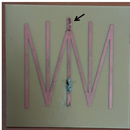
FIGURE 6.14: Adjusted folded comb-line prototype
