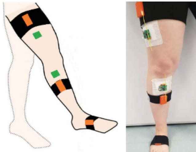
FIGURE 2.15: Sensor locations for Xsens and RFID units [79].
