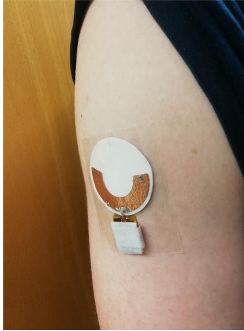
FIGURE 3.12: DDRR tag placement on the upper right arm attached via double sided tape.
