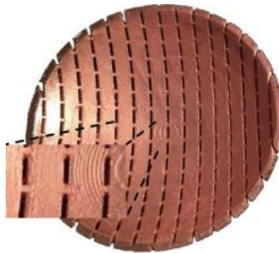
Figure 2.18 A self-supporting 3D printed conformal FSS with the settings after metallization of the optimized print [150].
