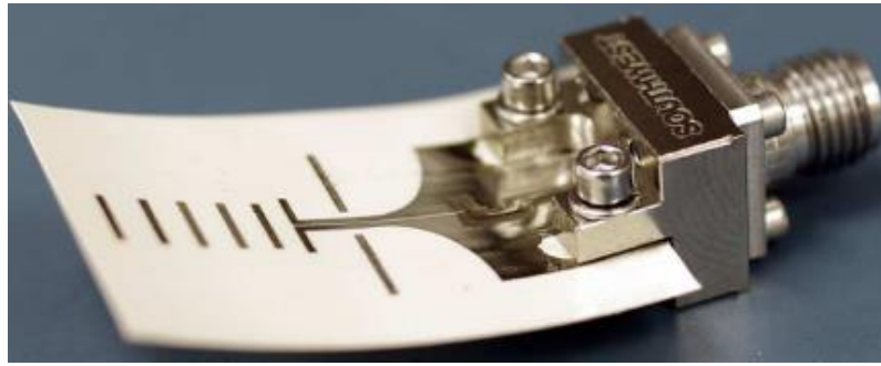
Figure 2.8 Inkjet-printed multilayer 5-director Yagi–Uda antennas with the printed dielectric substrate for the microstrip-to-slotline feeding transition [75]
