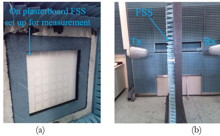
Figure 6.28 The FSS on the plain wave screen (b) chamber the measurements set up
