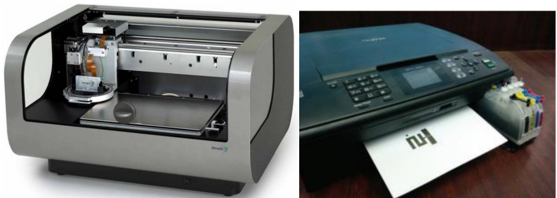
Figure 2.10(a) Dimatix DMP 2800 inkjet printer [92] [93] and (b) Brother inkjet printer with a printed antenna [94]
