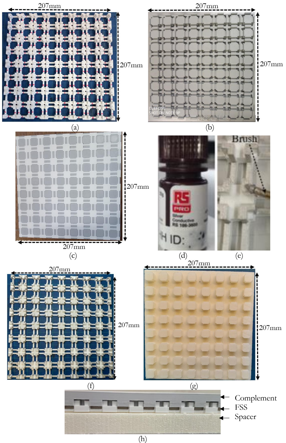
Figure 6.15 The (a) printed FSS substrate, (b) substrate complement (c) FSS and complement locked together (d) RS pro Silver Conductive 186-3600 paint (e) brush painting the FSS (f) painted FSS (g) foam spacer (h) side view of spacer positioning the complement
