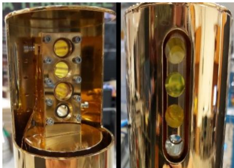
Fig. 4.2: Photographs of the sample holder with its heat shield as seen from the front ( left ) and rear ( right ) sides. In these photographs, three ZnSe substrates are mounted onto the sample holder with the fourth position being used as a 9.6 mm diameter collimator. This collimator, along with a Faraday cup positioned opposite to an incident charged particle beam, allows for the determination of beam homogeneity.
