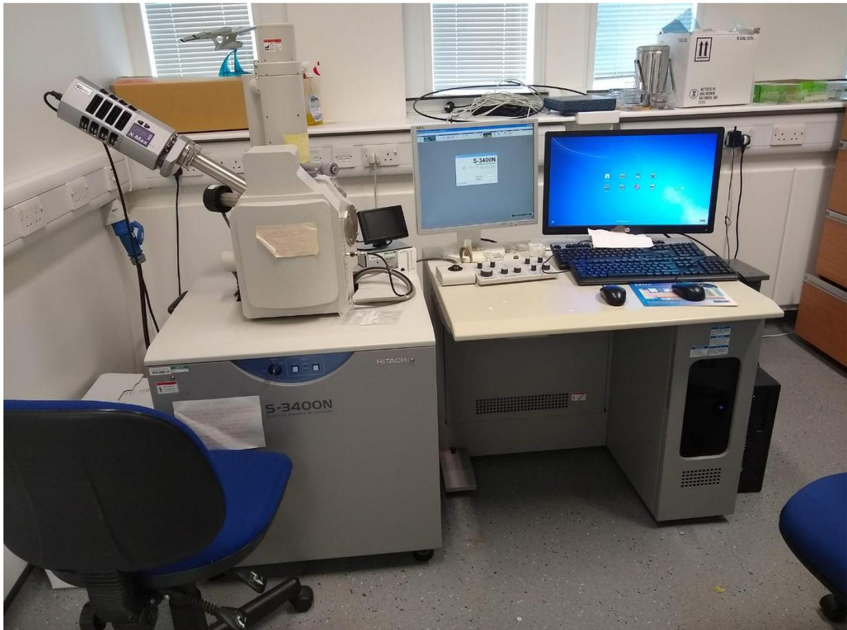
*Figure 2.8. Image of the Hitachi 3400N SEM with an Oxford Instruments 80 mm<sup>2</sup> X-max Energy Dispersive X-ray Spectrometer at the University of Kent.*
