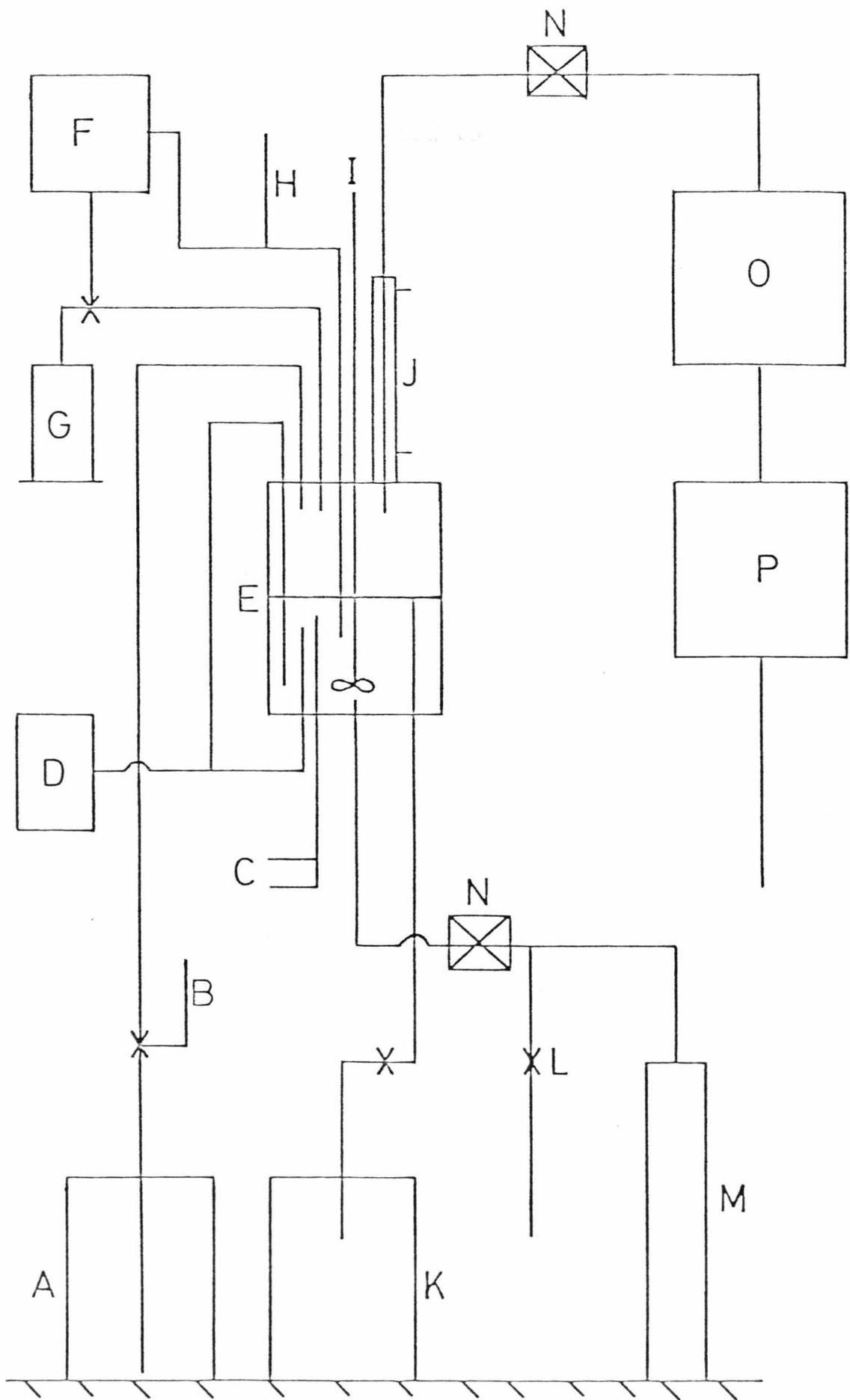
Temperature control was provided by a pulse ratio controller (Nobel Instruments Ltd.) using a 180 W, 240 V heating cartridge in conjunction with a cooling finger using circulating water at 10°C.
