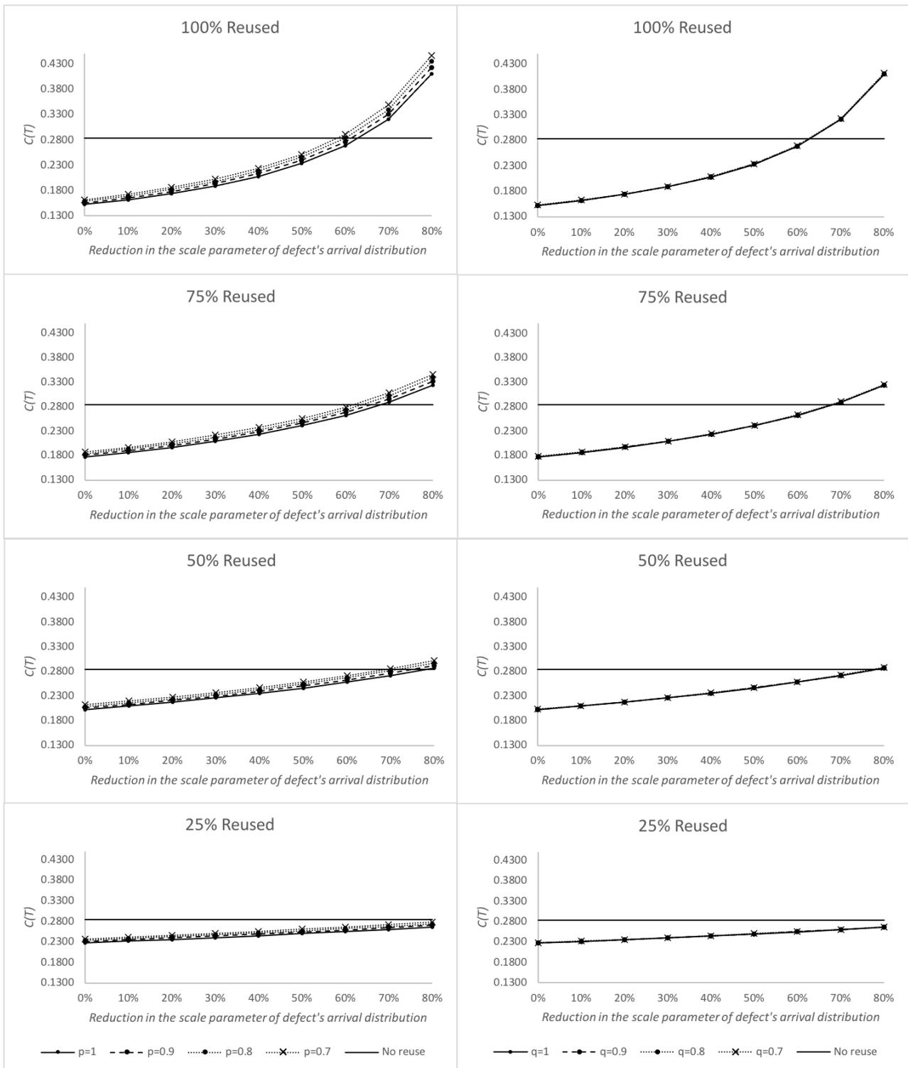
**Figure 7.** Effect of misclassification on the optimal inspection interval. On the left, variation on the probability of misclassification of minor defects. On the right, variations on the probability of misclassification of major defects.
