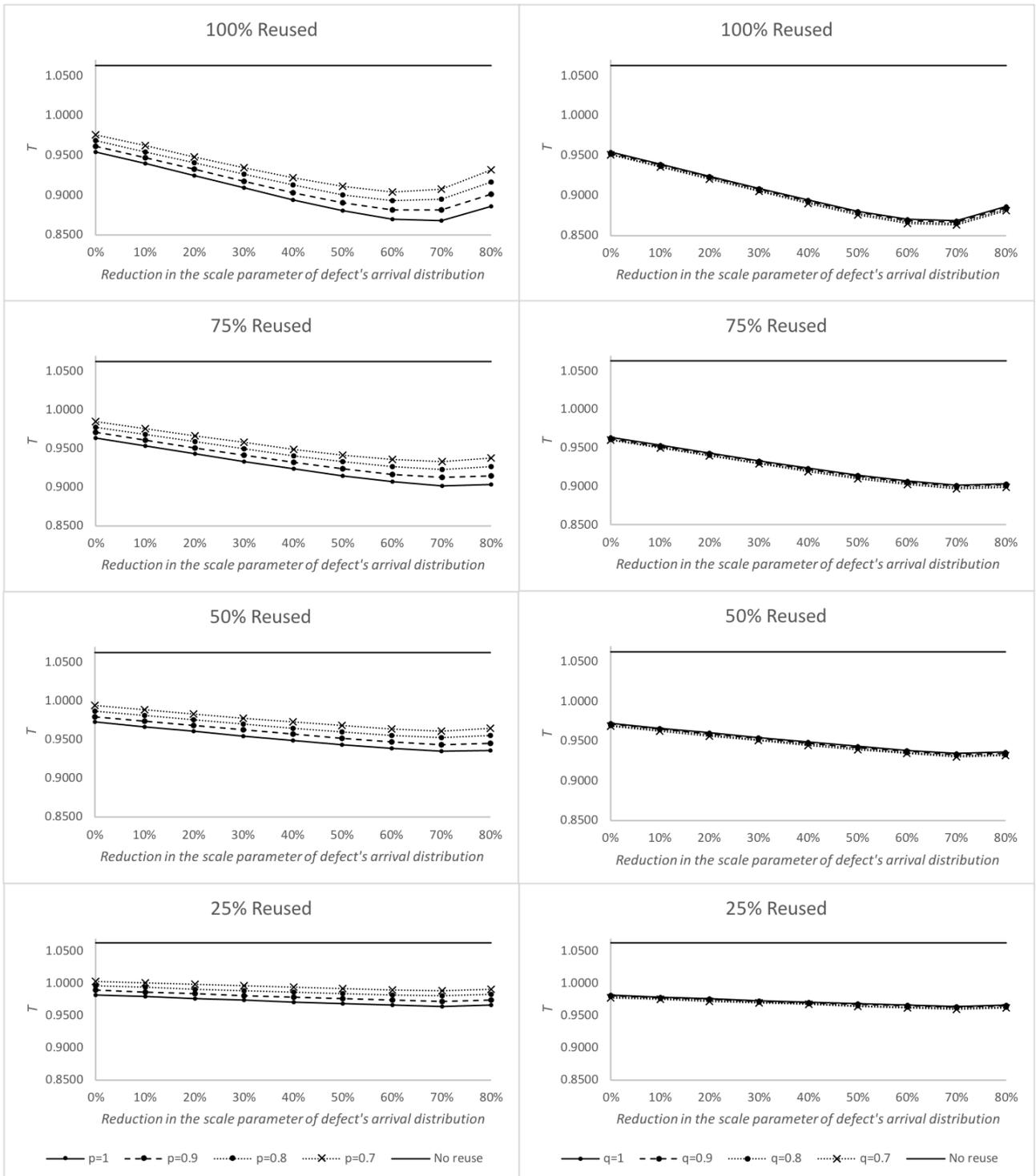
**Figure 6.** Effect of misclassification on the optimal inspection interval. On the left, variation on the probability of misclassification of minor defects. On the right, variations on the probability of misclassification of major defects.
