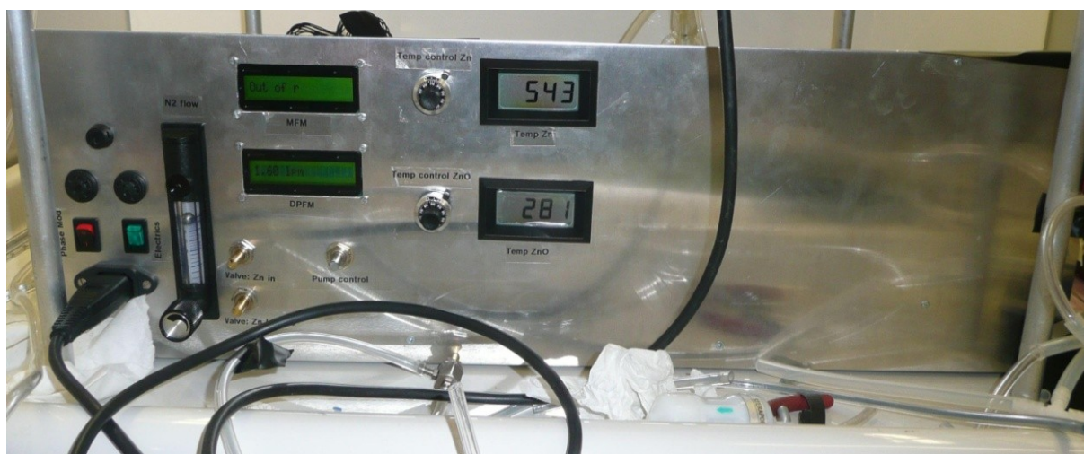
Figure 4.2–3. ZnO Generator front panel.
