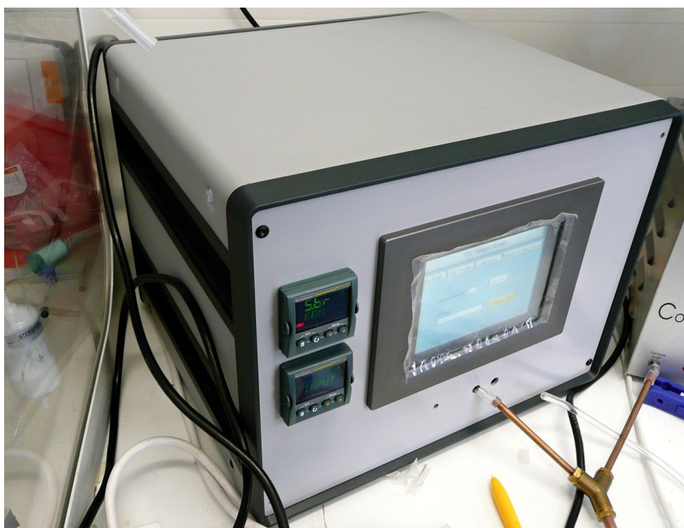
Figure 4.5-4. Surface area prototype instrument during testing. The y-splitter visible at the inlet is providing an equal aerosol split between the prototype instrument and in this case a Grimm CPC at the edge of the field of view to the right. The condenser temperature is controlled by the temperature controllers to the left of the main screen whereas the saturator temperature is controlled via the main software interface operated through the touch panel.
