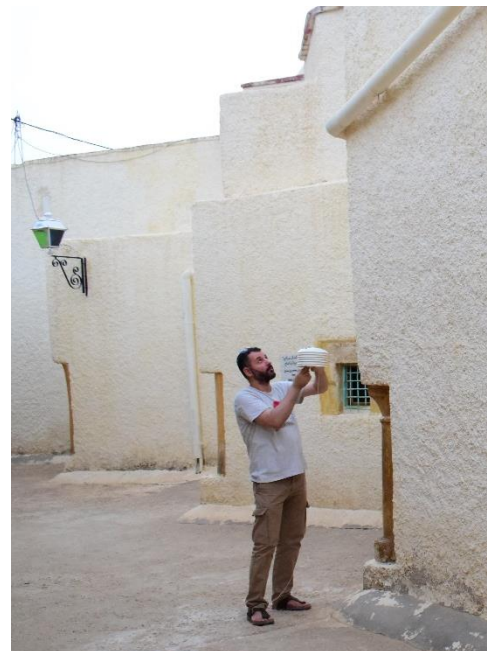
Figure 4.1 A HOBO data logger was placed outside of Beni Isguen houses (source: by the Author).
