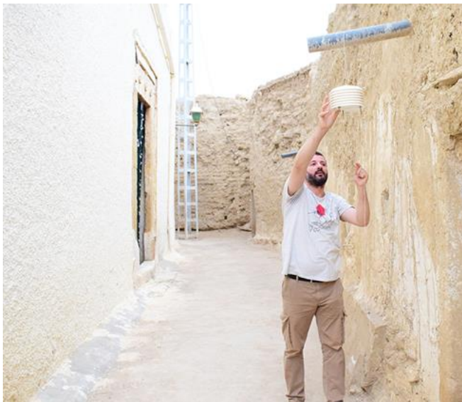
Figure 4.3 data logger was installed at a height of 2.5 metres above the ground (source: by the Author).
