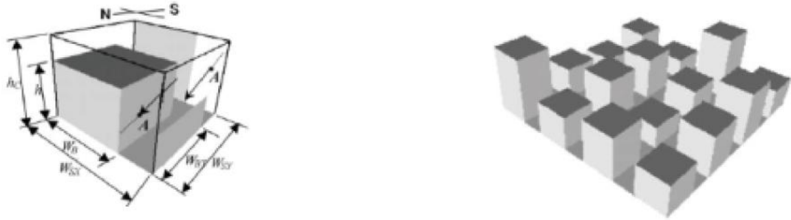
Figure 2.9 Left: the square-shaped building model used for the digital study. Right: the second study configuration with differentiated heights (source: Kondo et al. 2001).
