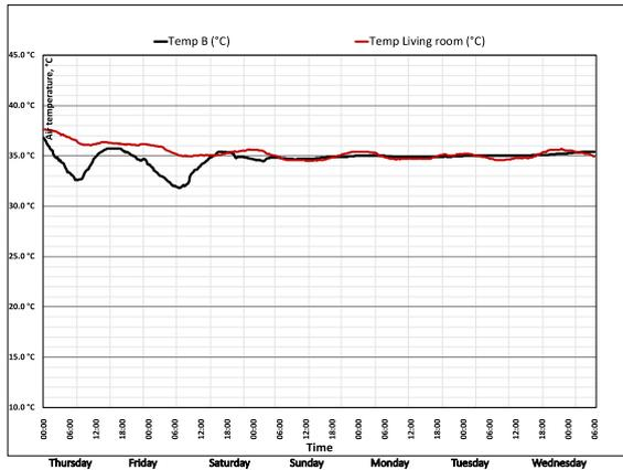
Figure 8: Comparison of the air temperature for outdoors and a living room in location B for one week
