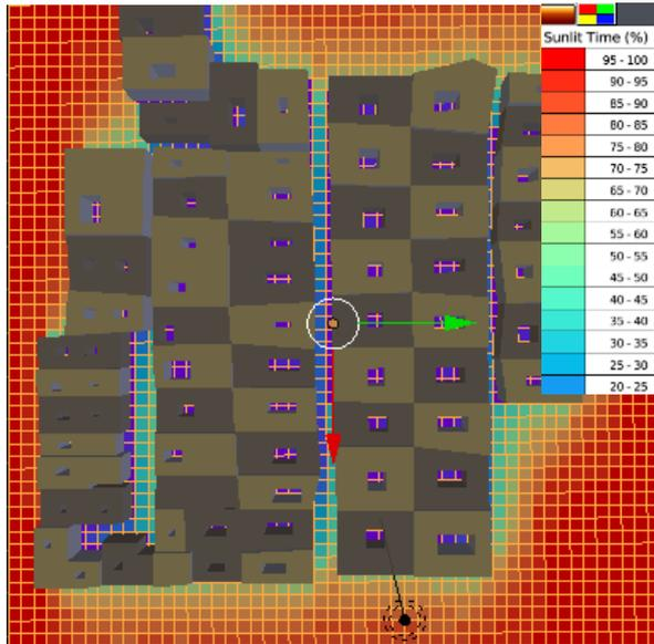
Figure 12: Shadow mapping for Beni Isguen
