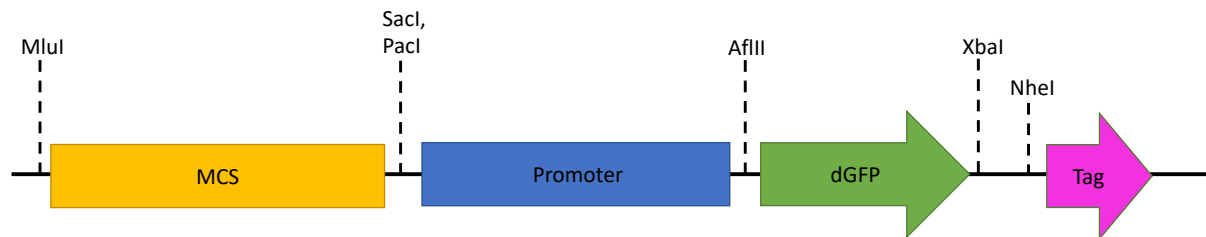
Figure 3.13 Schematic of plasmid layout with key restriction sites present. Between critical points of the DNA strand were placed restriction sites the user can utilise to insert the desired segments of DNA. The above sites are highlighted to visualize how the cloning was planned and performed in this study.
