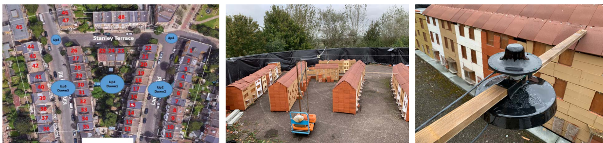
Figure 2 Left: the case study area in Islington, London; Middle: the 1:10 scaled model developed with real building materials; Right: pyranometers taking incident and reflected radiation measurements at canyon eaves level using IR filters and shade
