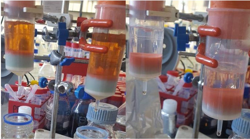
Figure 5.2 Immobilised BtuG on Ni 2+ - sepharose columns, trapping HBAD-like B 12 intermediates. ED661 cell lysate was loaded onto BtuG-columns (left), and bound HBAD (right).
