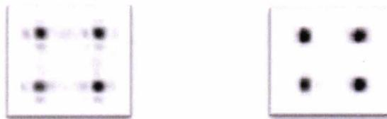
Fig. 6.29. Comparison of CG/SH-WFS spots without (left, MLA300-14AR ) and with (right, MLA150-5C) chrome apertures; these two images were acquired with TD-Cg/SH-WFS method.
