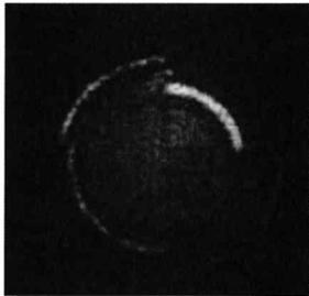
Figure 4.9 *En-face* coherence image obtained with the MDE inserted in the reference path.
