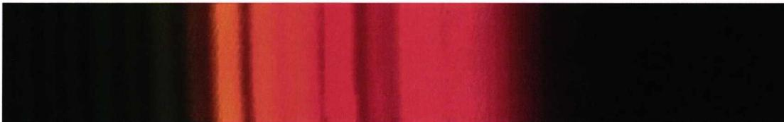
Figure 5.24. Spectrum image acquired using the Xenon flash lamp as the light source and the Canon 50D DSLR as the detector array in LF-FD-OCT.
