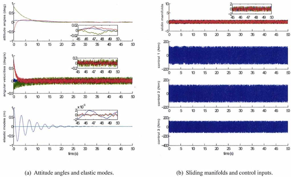
FIGURE 9.1: SMC: using  $\text{sign } u_i(t)$  with a varying delay  $\mu\xi(t) \leq 0.01s$ .
