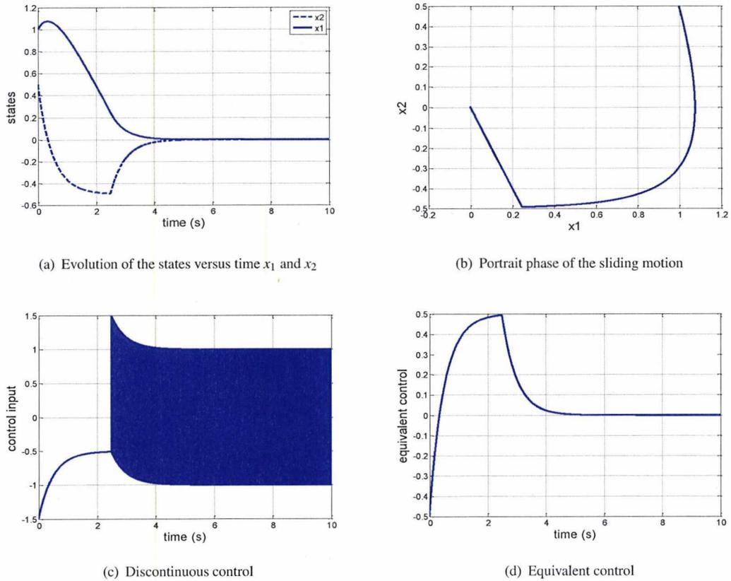
FIGURE 2.7: Sliding mode control (2.27) of system (2.26)
