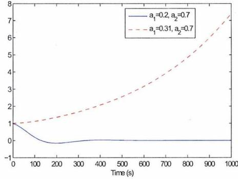
FIGURE 4.4: Response of system (4.36) with  $h_1 = 2s$ ,  $h_2 = 5s$
