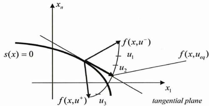
FIGURE 2.6: Sliding mode equation by Equivalent control method (Utkin, et al., [138], 2009)
