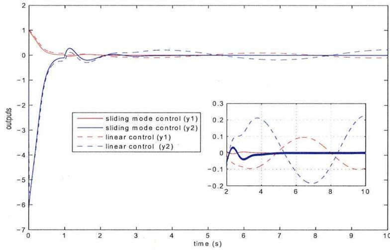
FIGURE 8.3: Comparison between sliding mode control and linear control in the presence of matched disturbance a
