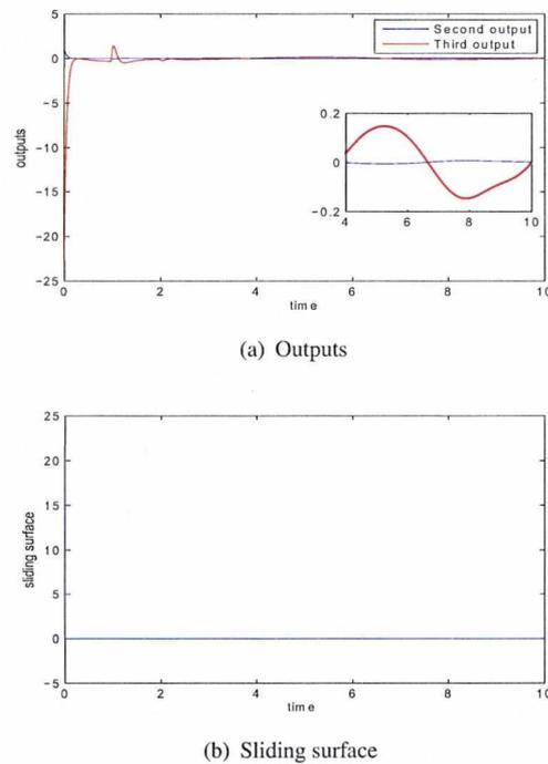
FIGURE 8.1: Closed-loop response with delay  $h = 1s$
