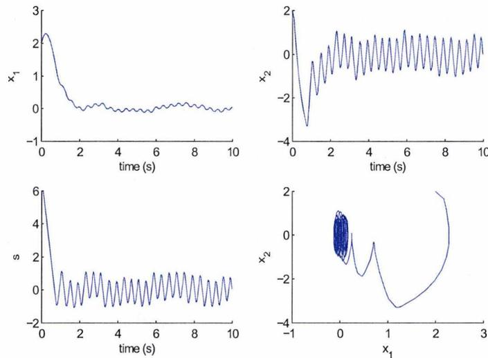
FIGURE 5.1: system (5.42) with control (5.43), designed without care of a delay  $\tau = 0.1s$ . (Figures are generated using Simulink ode1(Euler) solver with fixed-step size 0.0001s)
