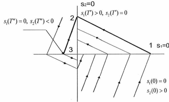
FIGURE 2.3: Sliding mode in the system with two-dimensional control (Utkin, et al., [138], 2009)
