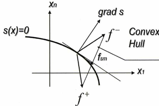
FIGURE 2.5: Sliding mode equation by Filippov's method (Utkin, et al., [138], 2009)
