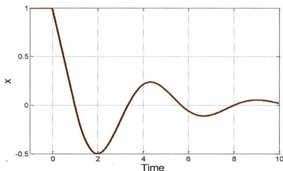
FIGURE 4.1: System  $\dot{x}(t) = -x(t-h)$  with  $h = 1$ ,  $\phi = 1$
