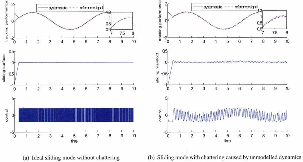
FIGURE 2.8: Sliding mode control of system (2.28)
