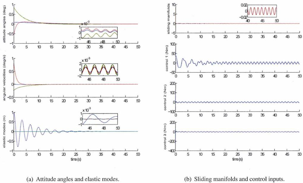
FIGURE 9.2: SMC: using smooth approximation of  $\text{sign } u_i(t)$  with a varying delay  $\mu\xi(t) \leq 0.01s$ .
