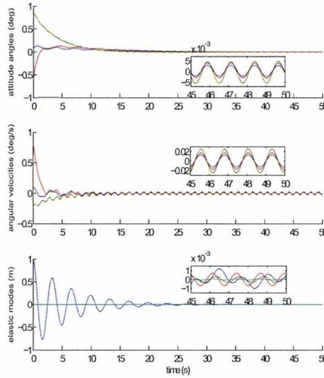
FIGURE 9.3: Linear control: Attitude angles and elastic modes with a varying delay  $\mu\xi(t) = \mu\xi(t) \leq 0.01s$ .
