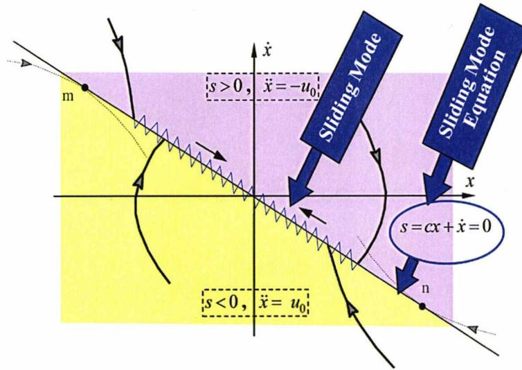
FIGURE 2.1: State plane of the second-order relay system (Utkin, et al., [138], 2009)
