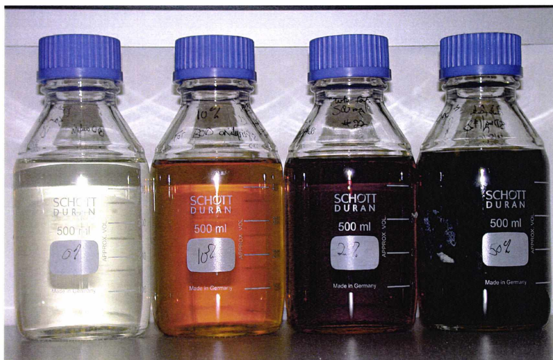
Figure 7.5. Colour development in solutions of compound #22 after 120 min of photo-Fenton treatment showing increasing colour with increasing strength of treatment. Treatment (from left to right): 0%, 10%, 25% and 50% of ThOD.
