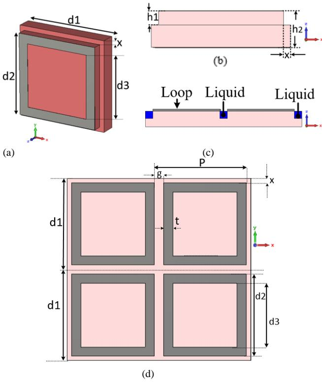
Fig. 1 shows (a) the perspective view (b) the cross-sectional view (c) cross sectional view of a section of the FSS sensor liquid-filled trenches (d) the top view of the unit cell
