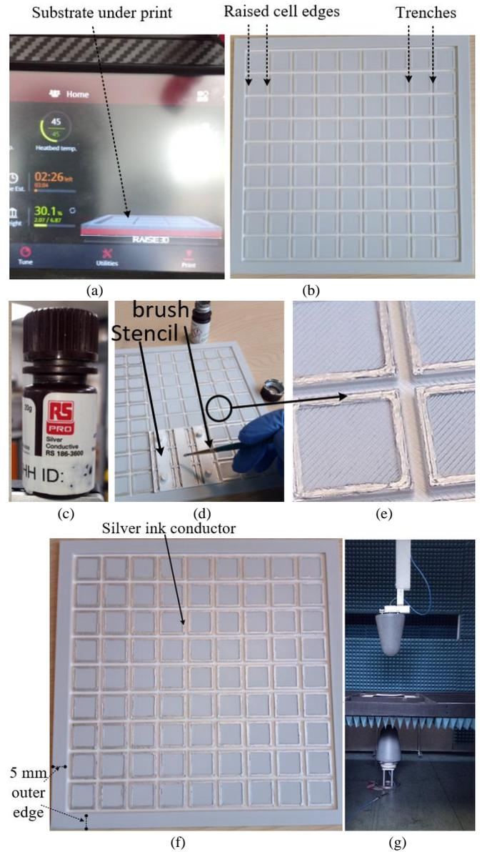
Fig. 4 The fabrication process of the 3D sensor (a) the printing of the substrate with a Raised 3D printer machine (b) the printed PLA substrate (c) the silver paint the printing of the substrate (d) applying silver loops (e) section of the painted FSS (f) the finished 3D FSS (g) the FSS sensor measurement setup.
