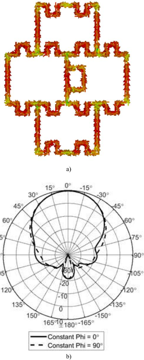
Fig. 5. Simulated pattern of current (a). Simulated radiation gain for the meandered 4-cell wearable GAA (b).
