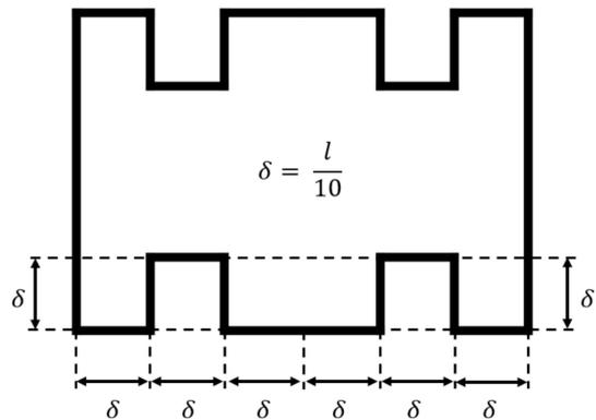
Fig. 4. Meandered GAA Cell
