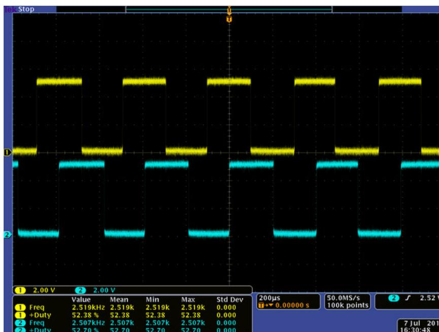
Figure B.3: Outputs of encoder channel A and B when the motor runs at 12V
