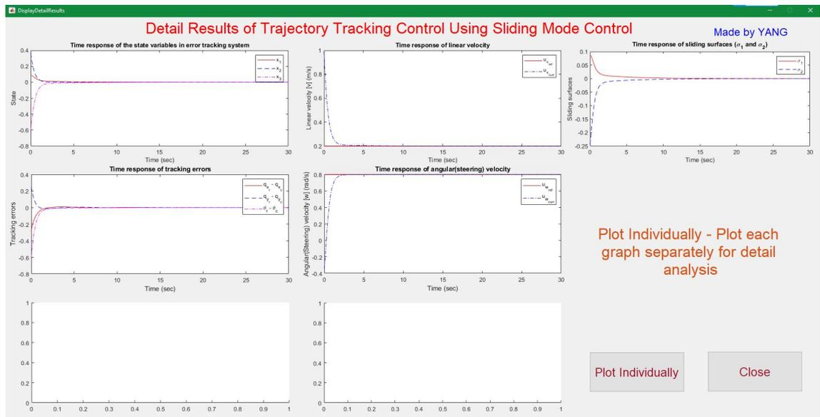
Figure C.2: Details information of the trajectory tracking control on a TWMR system under Matlab simulation
