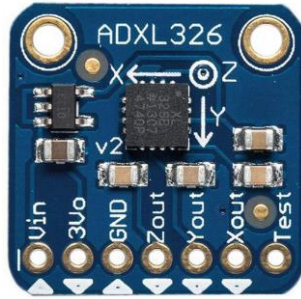
Figure 3-7: Interface diagram of the ADXL326 accelerometer [68].
