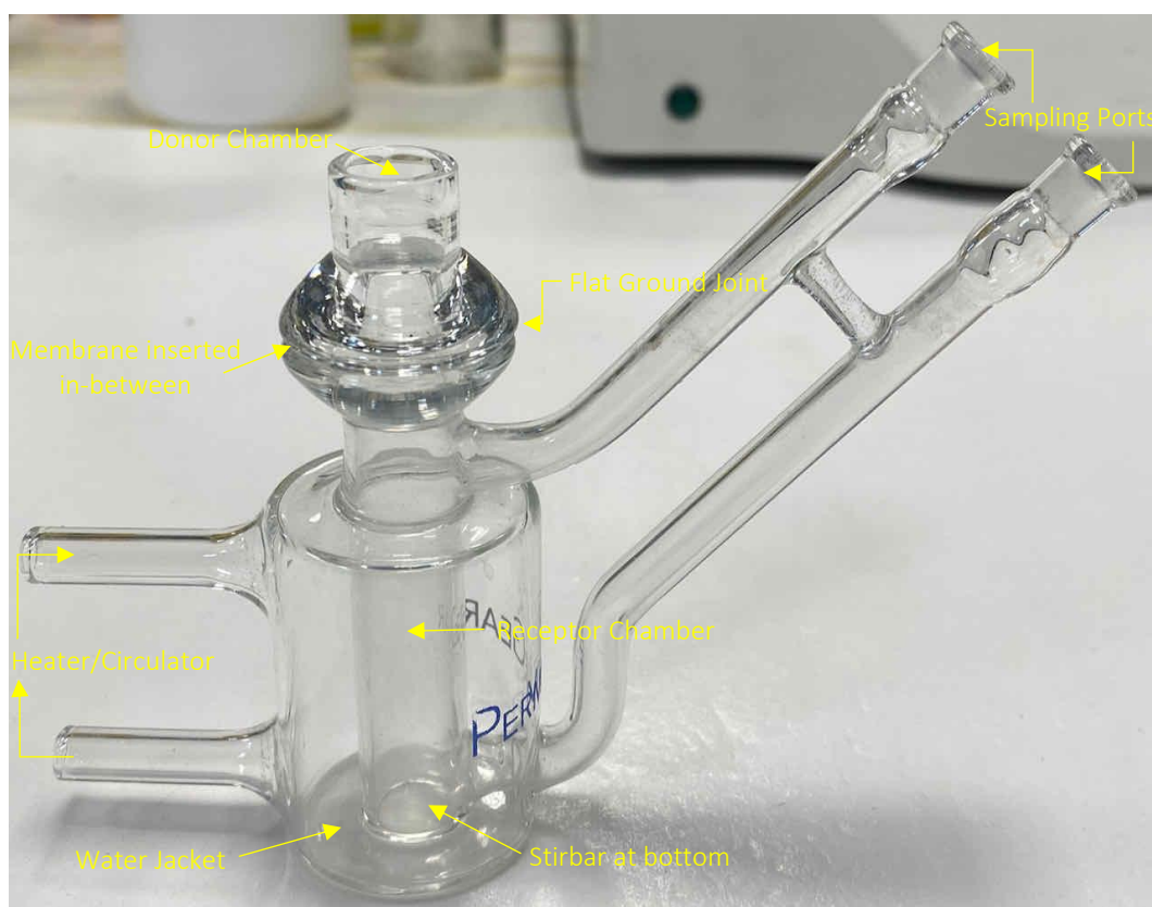
Figure 63 Labelled image of a Franz Diffusion Cell - the skin (membrane) is inserted between the donor chamber and receptor chamber before they are filled with solution
