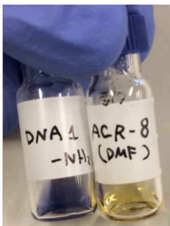
Figure 4.6. Kaiser test results for DNA1-NH 2 control (left) and ACR-8 (right). The result was negative in ACR-8 , confirming the absence of primary amines.
