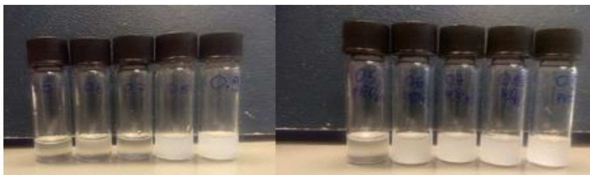
Figure 202 Polymer dispersions in THF: Water (Left)- PEO 16 -b-PBMA 10 and (Right)- PEO 12 -b-PBMA 10
