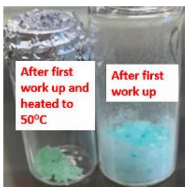
Figure 160 (Right) Sample of PMMA-Br after the first purification stage showing blue polymer indicating copper leakage. (left) Sample of PMMA-Br after first purification stage after it had been in the oven for at 80°C for an hour. Green colour indicating present of copper.
