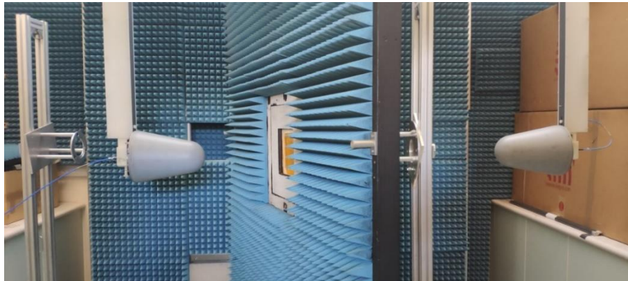
Fig. 6.19 Measurement setup for millimetre wave bandstop FSS designs
