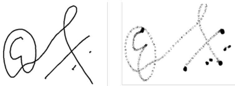
Figure 2.5. a) Static Signature (left) b) Dynamic Signature (black dots represent pen-down and pen-up points) (right)
