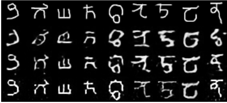
FIGURE 3.17: The figure shows the reconstruction results of 9 random selected Omniglot characters using the hardware measurements. The images at the top row are the original ground truth images, and the images from the second to the last row are reconstructed results at R = 0.01, 0.1 and 0.25 .
