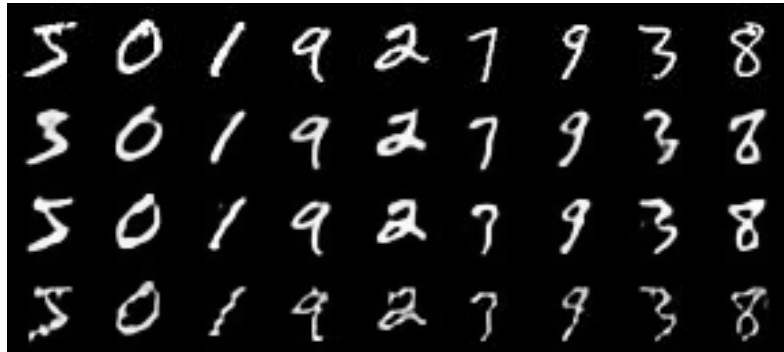
FIGURE 3.16: The figure shows the reconstruction results of 9 random selected MNIST handwritten numbers using the hardware measurements. The images at the top row are the original ground truth images, and the images from the second to the last row are reconstructed results at R = 0.01 , 0.1 and 0.25 .
