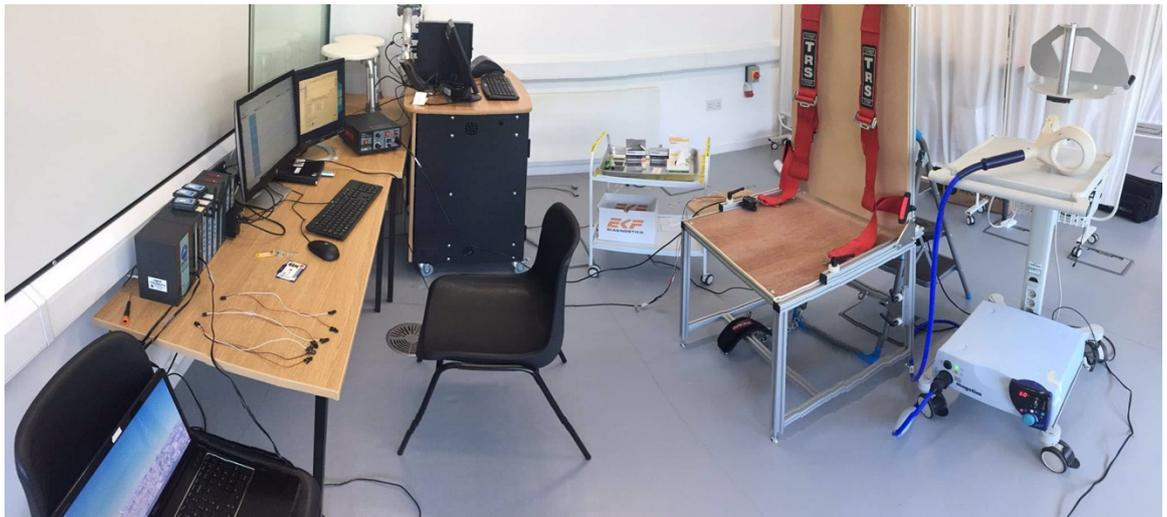
Figure 22. Image of the custom-built dynamometer used in Part B.
