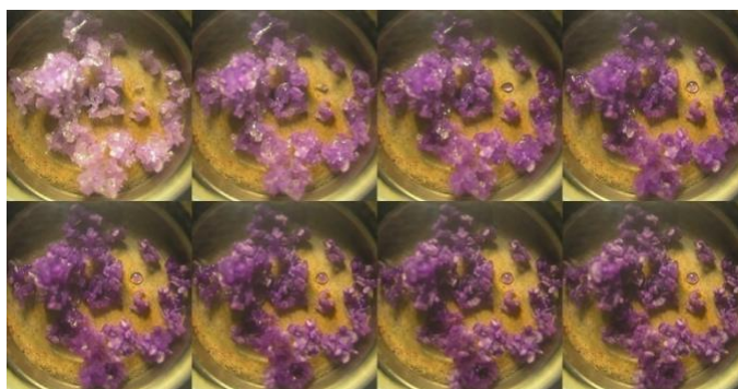
Figure 23: This reflectivity montage depicts the formation of [\text{Fe}(\text{atrz})_3]\text{SO}_4 over time immediately after mixing. The top left image can be assumed to be at zero seconds with the bottom right image at 3000 s.
