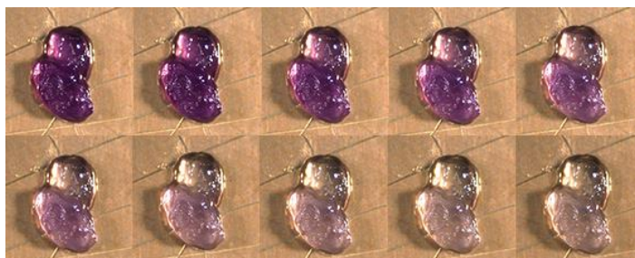
Figure 22: Single crystal reaction heated from 298 K to 373 K to determine crossover capability. The first image (top left) was taken at 298 K and the last image was taken at 373 K. As this was preliminary testing to see if it switched, individual temperatures were not acquired.
