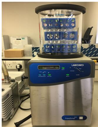
**Figure 7.2. Labconco™ FreeZone™ 2.5L freeze drier.** The machine is comprised of a freezer lowering the temperature in the top chamber, and an attached pump (left) that creates a vacuum in the top chamber lowering the pressure. Inside the chamber there is a stack of 88 PV samples being freeze dried.
