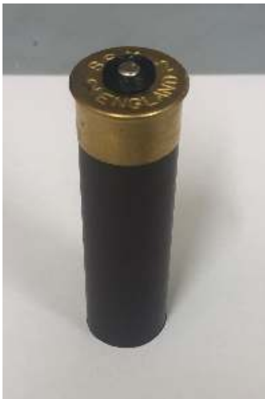
Figure 7.6: Picture of the fully modified CCI 10 shotgun cartridge with the CCI Mini-Mag primer loaded using the 3D printed adaptor.
