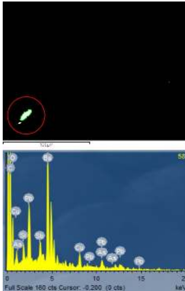
Figure 4.10: BSE SEM/EDX binary image and spectrum of a ‘unique’ GSR particle using the INCA GSR automated software, showing an example of the irregular, non-spheroidal morphologies encountered during the particle identification process. This particle is approximately 14 \mu\text{m} in diameter and was found 40 cm from the firearm. HV : 27 kV.
