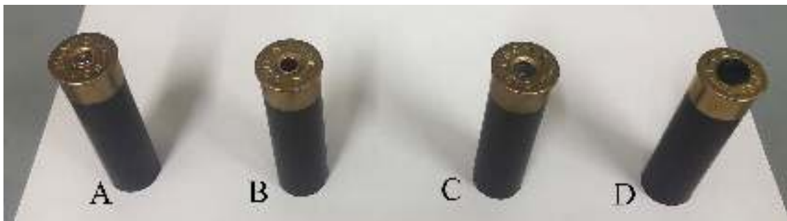
Figure 7.5: Pictures of the CCI 10 shotgun cartridge modification steps to include the primer adaptor. A: an original CCI 10 shotgun cartridge, B: the shotgun cartridge post primer firing, C: the shotgun cartridge with the primer cap removed, D: the modified shotgun cartridge containing the primer adaptor.
