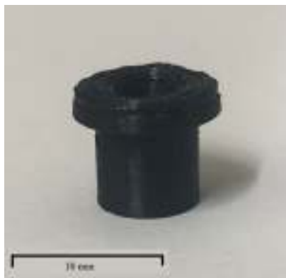
Figure 7.1: Picture of the 3D printed primer adaptor holder for CCI Mini-Mag primers that was designed by Vassilia Spathis (author) to fit into a CCI 10 shotgun cartridge.
