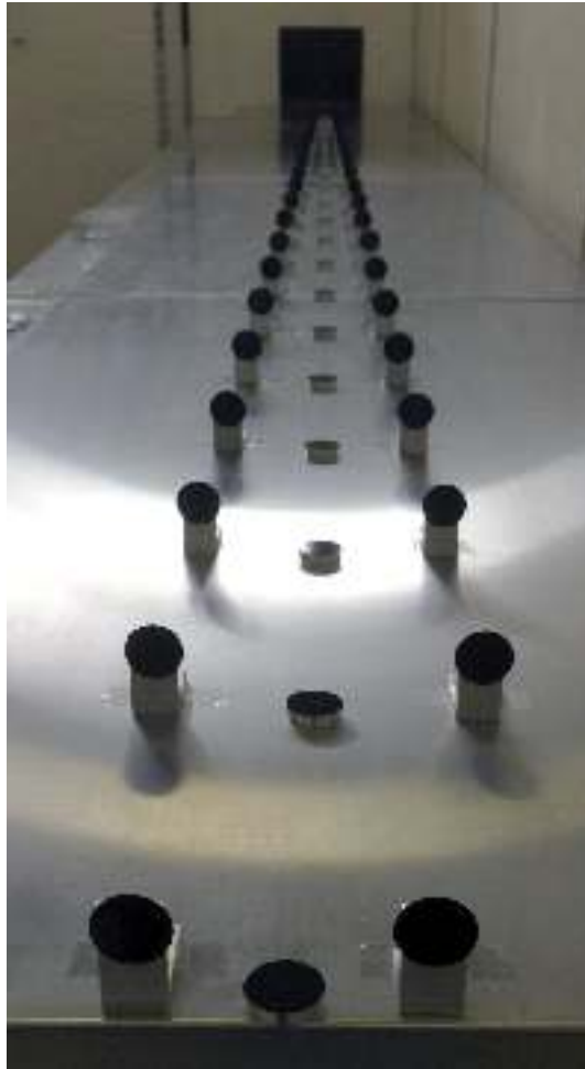
Figure 4.1: Photograph of the experimental set-up of Experiment 1.2 showing the decreasing sampling width along the entire 400 cm sampling range.
