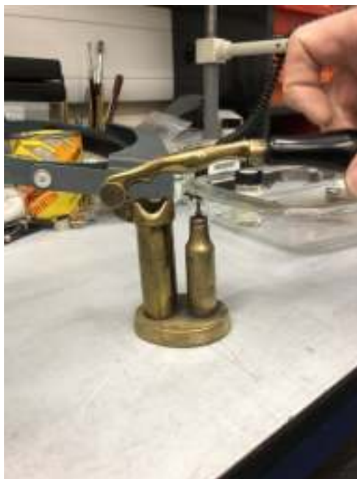
Figure 7.2: Picture of primer remover apparatus. Once the active primer was fired off on the LGG, the shotgun cartridge would be placed upside down with the pin sitting below the empty primer cap, allowing the cap to be removed and replaced by pushing the lever down.
