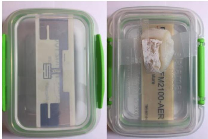
**Figure 2-26 – Perspective of the fish decomposition experiment from above (left) and below (right), where the RFID tag is adhered to the inside of the lid and the fish portion is taped down to the base of the container.**
