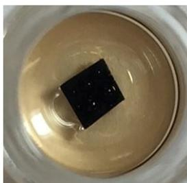
**Figure 2-18 – Photographs of MAF-5 suspended in a 1000 ppm diethylamine solution after 24 hours.**
