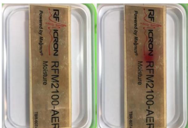
**Figure 2-29 – A comparison of the PDMS-MAF tag before (left) and after (right) addition of a single drop of concentrated ammonia solution.**
