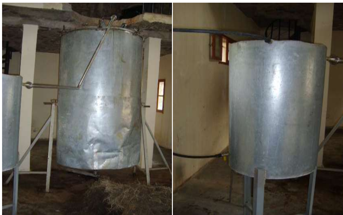
Plate 9.12: (a) The installed alembic with a capacity for 300 kilograms of plant material; (b) the condenser (El Maghzen, 2011).
