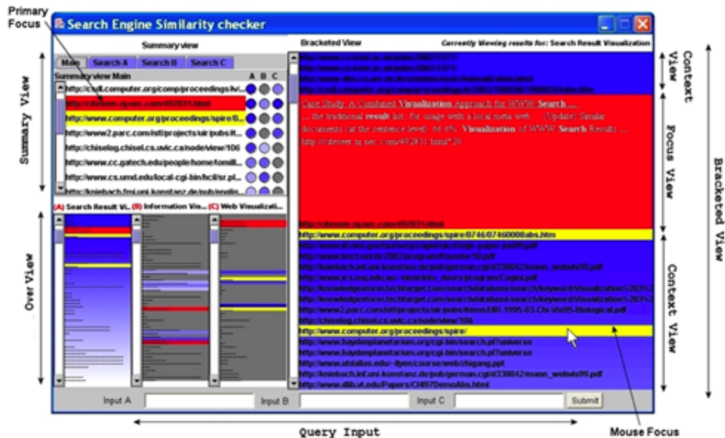
Figure 4.51: The SES (search engine similarity) tool. This contains four views, the summary view (top left), the overview (bottom left), and bracketed view (right). Users input queries in the bar along the bottom.
