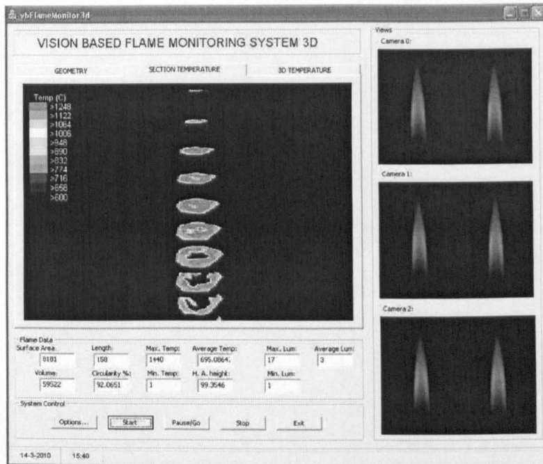
Figure 4.13: Software interface showing the second tab and the reconstructed cross-sections of temperatures.
