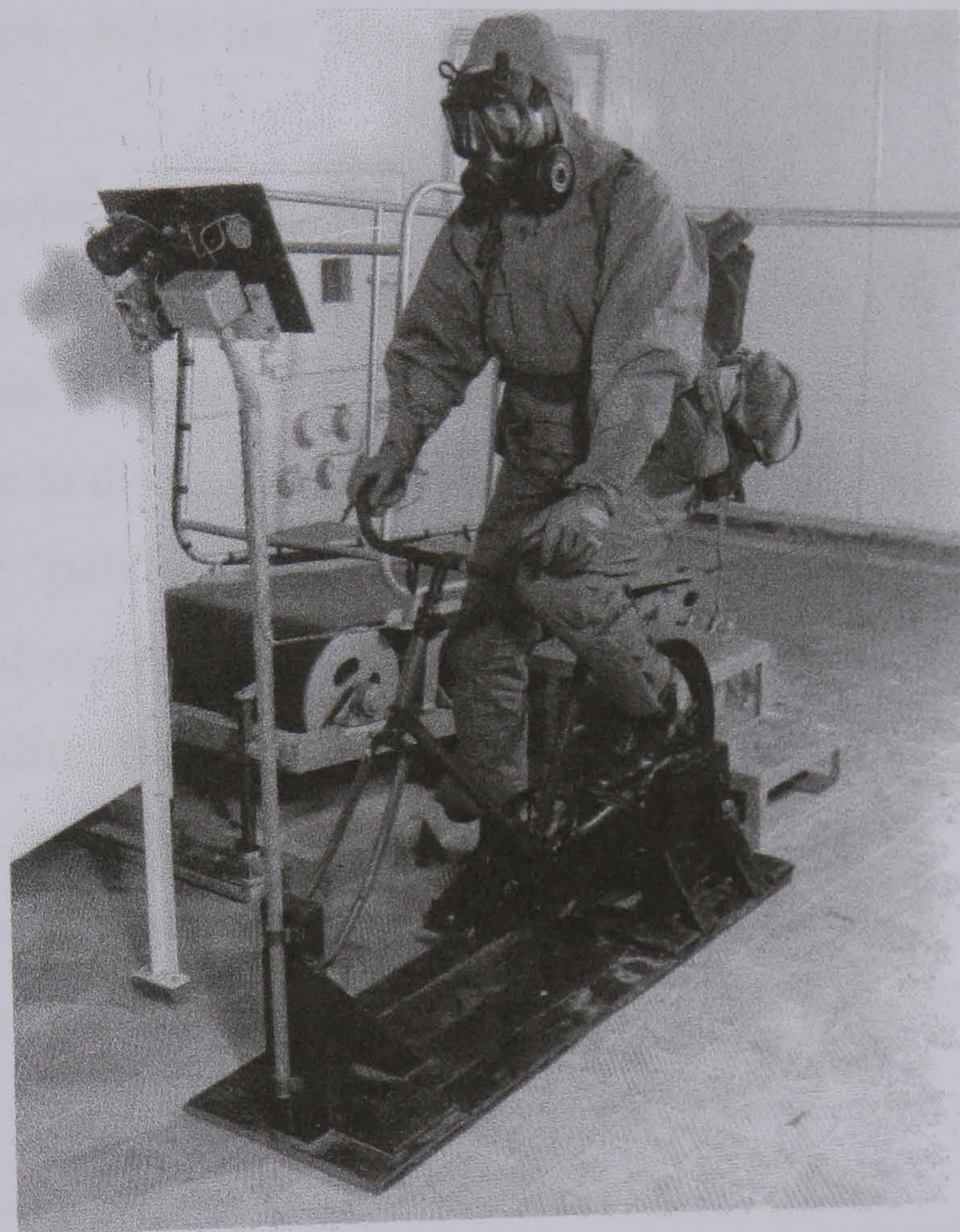
Figure 4 Testing of NBC suit at Porton, undated (photograph donated by Gradon Carter, Dstl, Porton).
