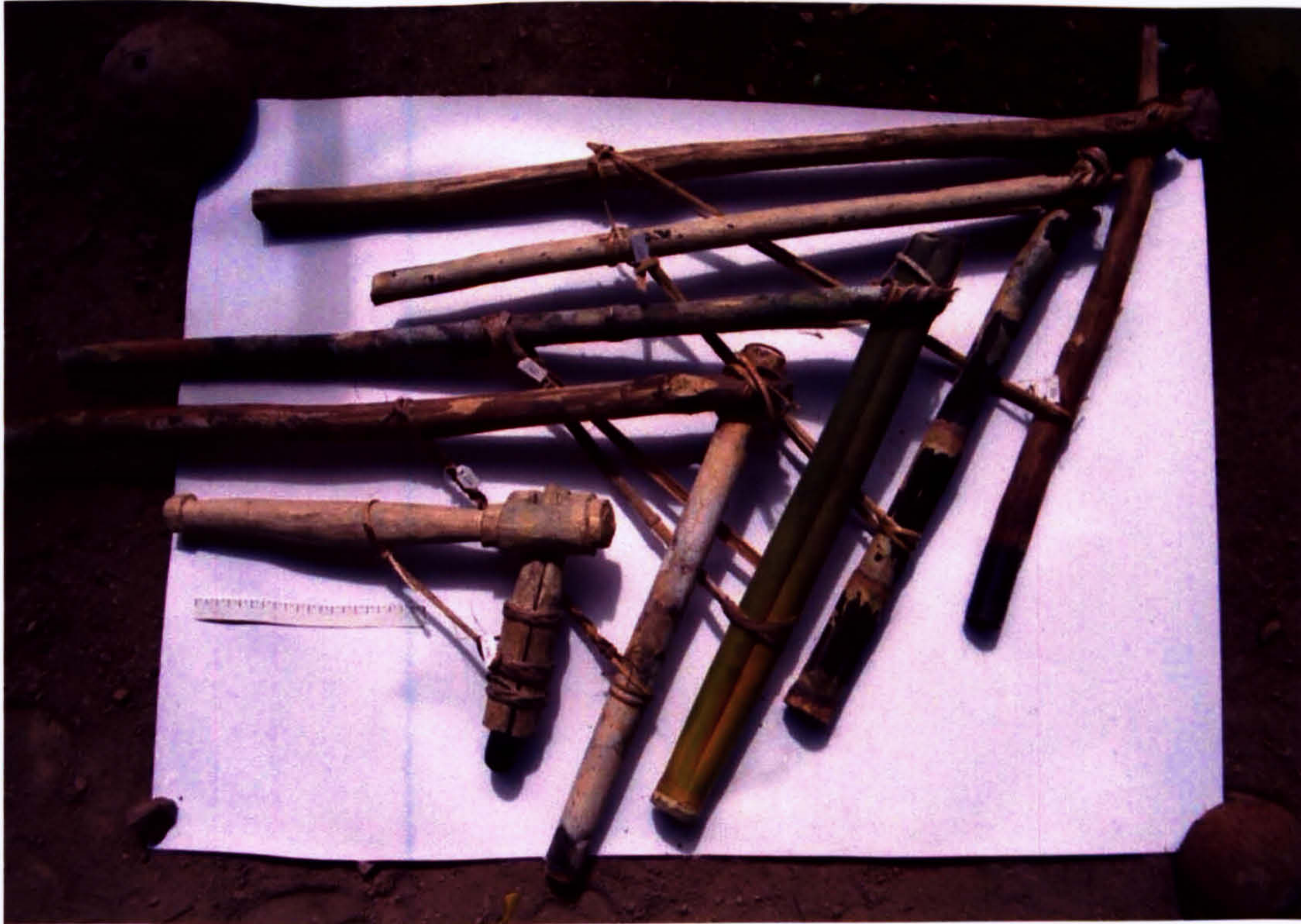
Plate 4: Sago Choppers. The image shows the entire spectrum of chopper designs used in Krisa (cf. Case Study 2). From left to right: reduced-size model of obsolete design with stone blade; designs with dry and green bamboo heads, the latter serving demonstration purposes only; design with rattan head; design with reinforced hardwood head.
